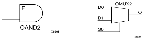
Figure 20: AND & MUX Symbols in XC4000X IOB
