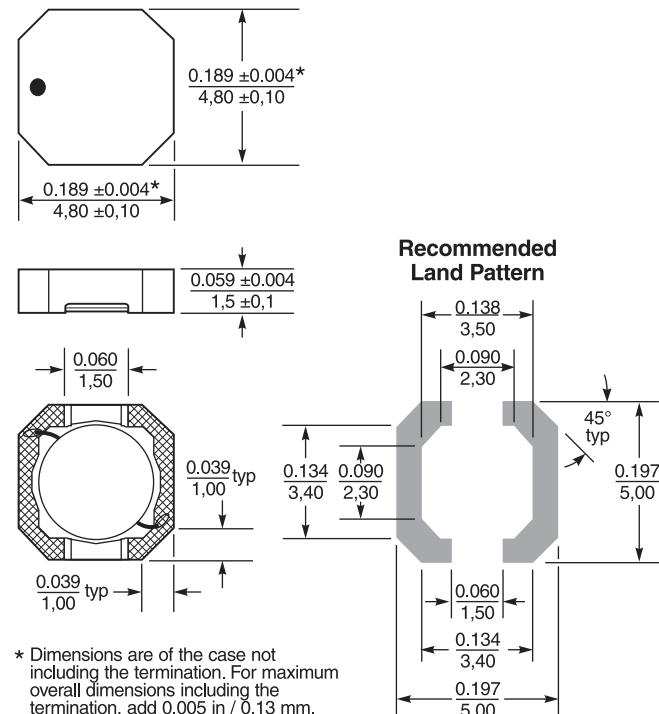
\* Dimensions are of the case not including the termination. For maximum overall dimensions including the termination, add 0.005 in / 0.13 mm.
