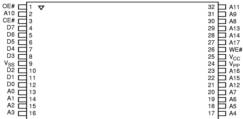
32-Pin TSOP—Reverse Pinout
