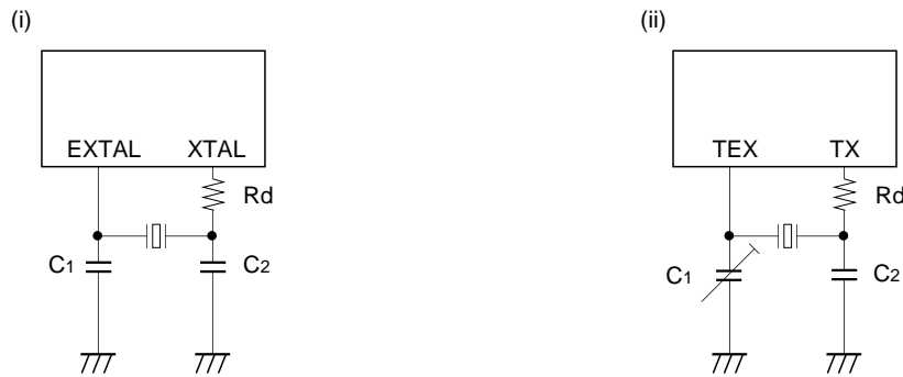
Fig. 10. Recommended oscillation circuit
