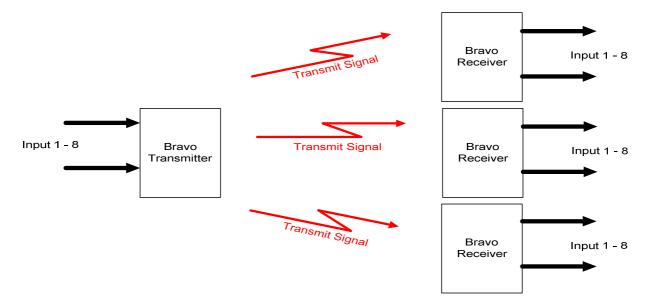
In this application the outputs at each of the receivers will track the inputs at the transmitter.
