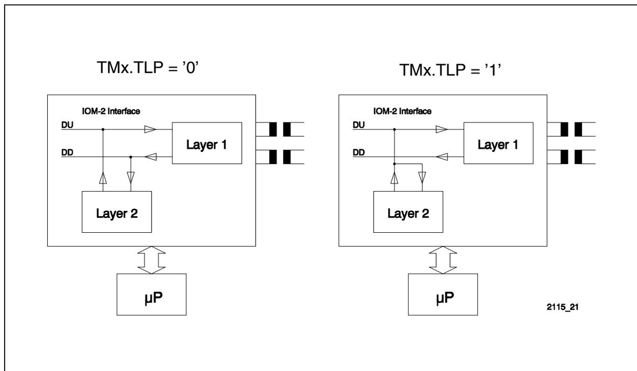
**Figure 109 Layer 2 Test Loops**
