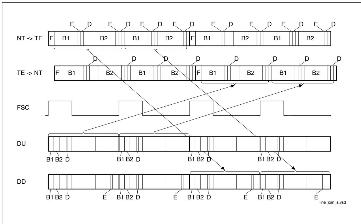
**Figure 56 Data Delay between IOM-2 and S/T Interface (TE mode)**
