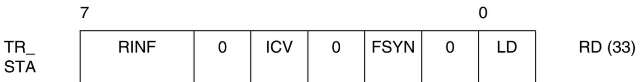
Important: This register is used only if the Layer 1 state machine of the SIUC-X is disabled (TR\_CONF0.L1SW = 1) and implemented in software! With the SIUC-X layer 1 state machine enabled, the signals from this register are automatically evaluated.
