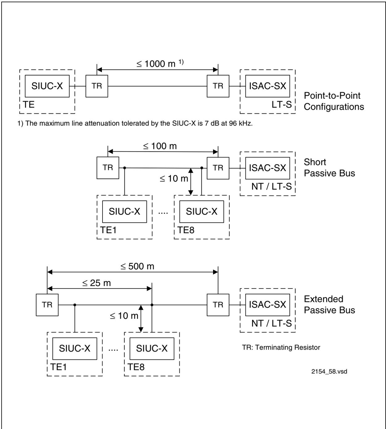
**Figure 51 Wiring Configurations in User Premises**
