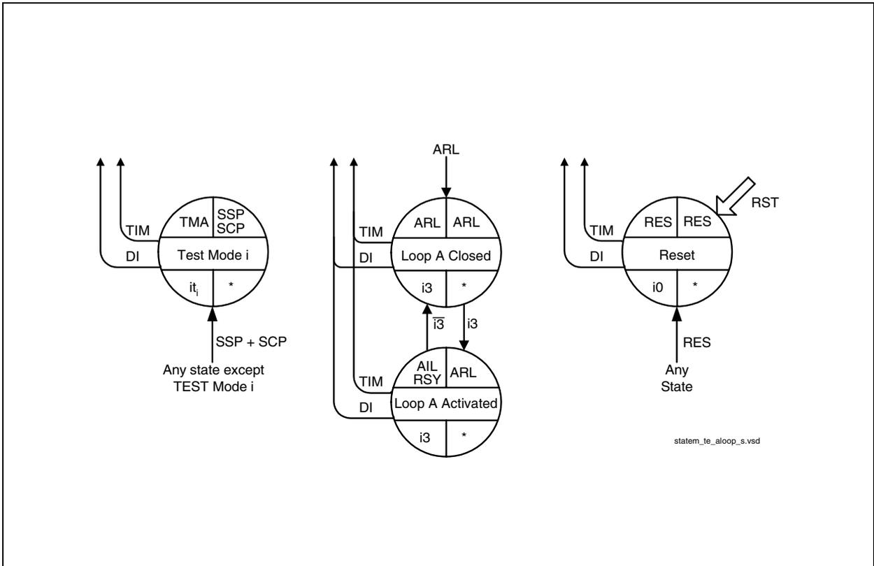
**Figure 68 State Transition Diagram of Unconditional Transitions (TE)**
