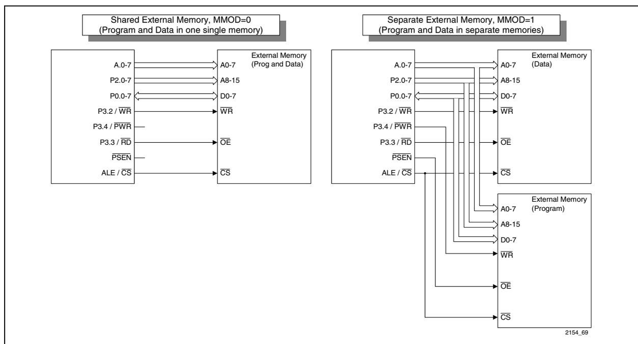
**Figure 118 Shared and Separate External Memory Expansion**
