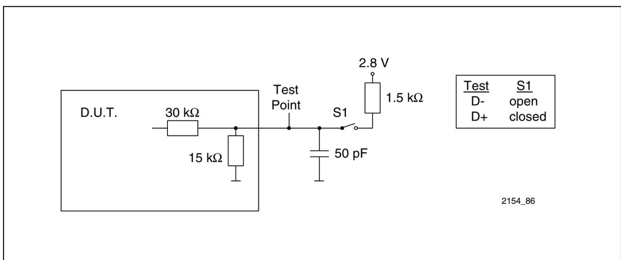
Figure 150 Load for D+/D-
