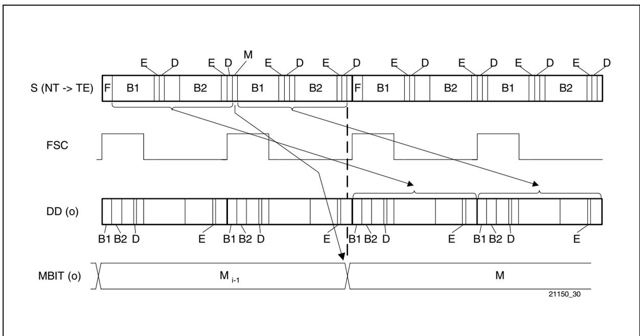
**Figure 55 Frame Relationship in TE mode (M-Bit output)**
