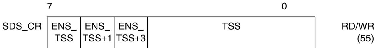
This register is used to select position and length of the strobe signal. The length can be any combination of two 8-bit timeslot (ENS\_TSS, ENS\_TSS+1) and one 2-bit timeslot (ENS\_TSS+3).
