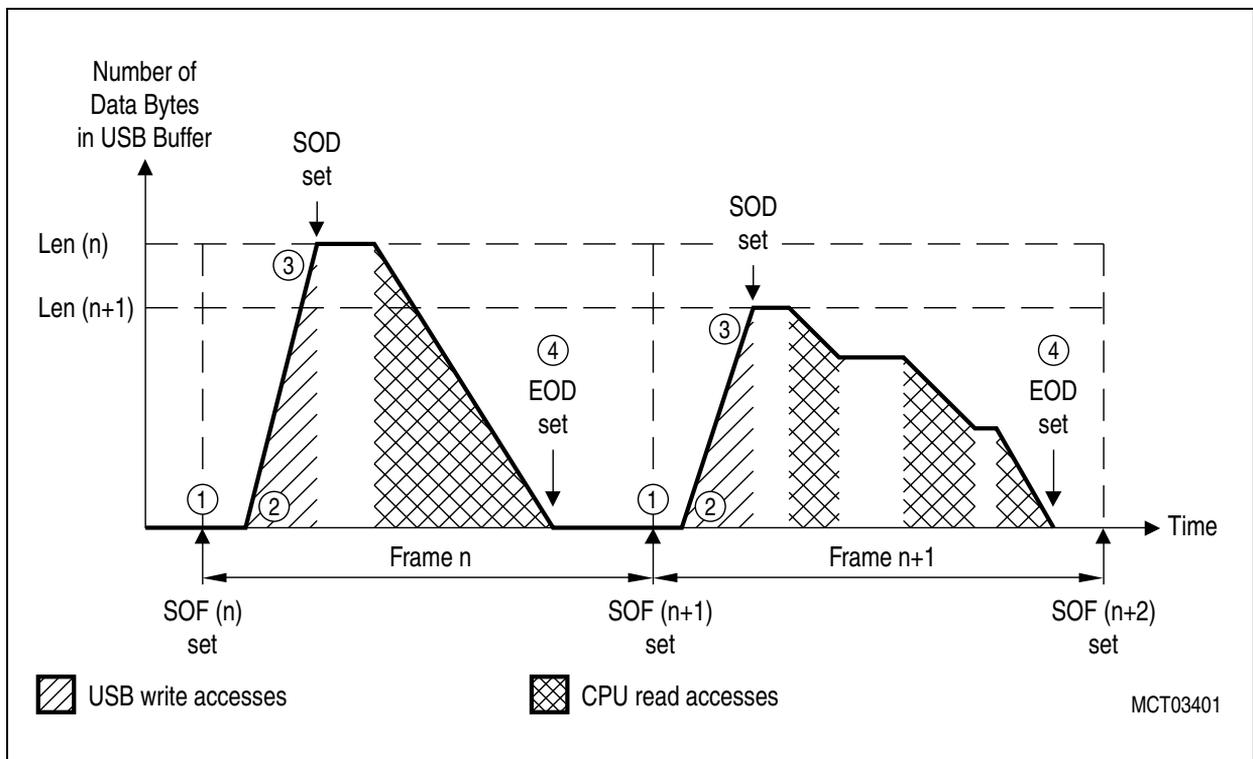
**Figure 27 Single Buffer Mode : Standard USB Write Access**
