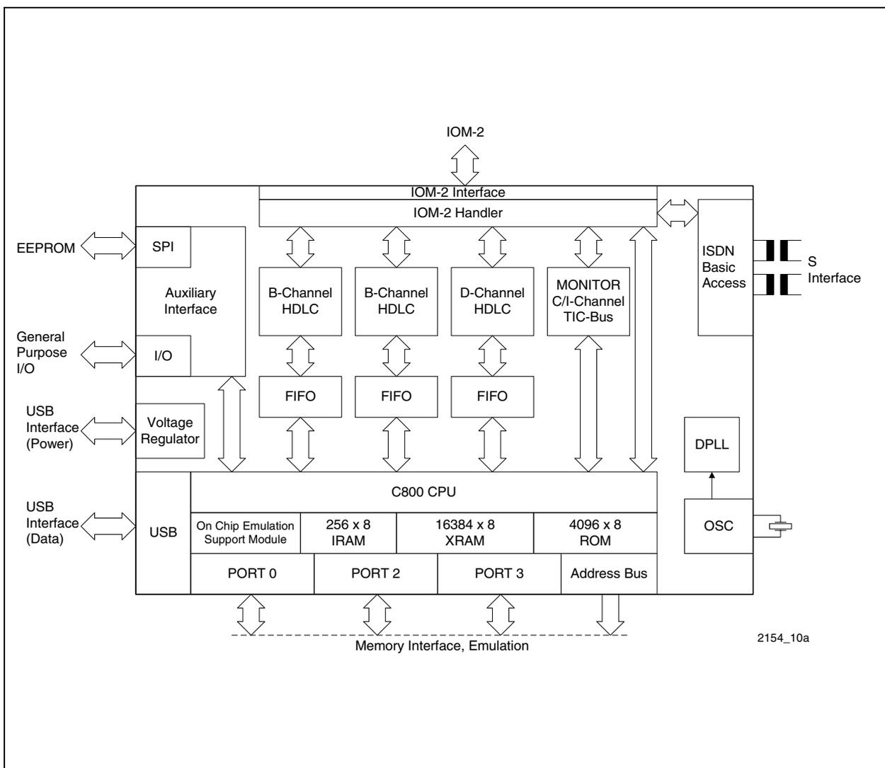
Figure 6 Block Diagram
