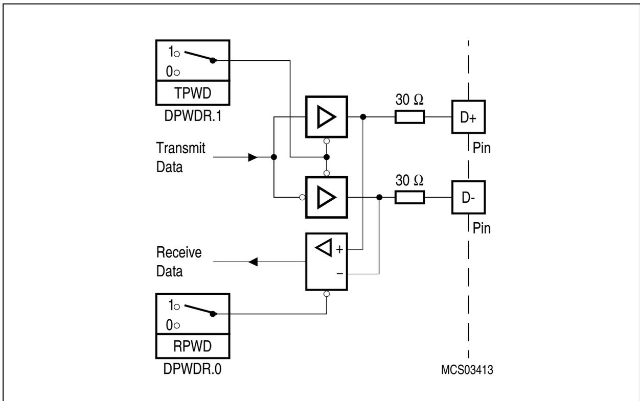
**Figure 39 USB Onchip Driver Circuitry**
