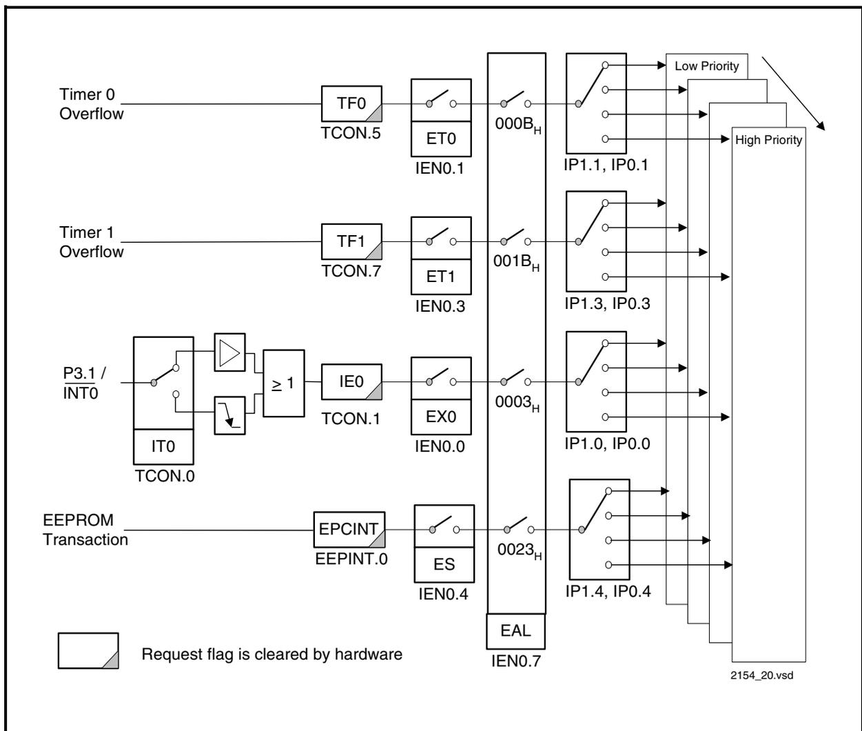
**Figure 111 Interrupt Request Sources (Part 1) - Miscellaneous Interrupts**
