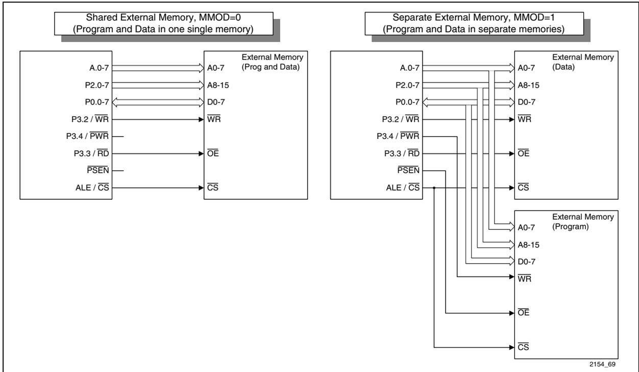
Figure 11 Shared and Separate External Memory Expansion
