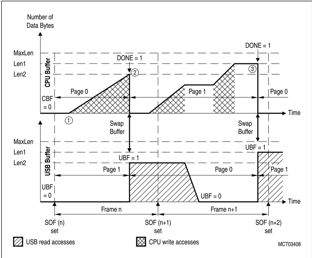
**Figure 34 Dual Buffer Mode USB Read Access: Buffer Switching by Setting Bit DONE**
