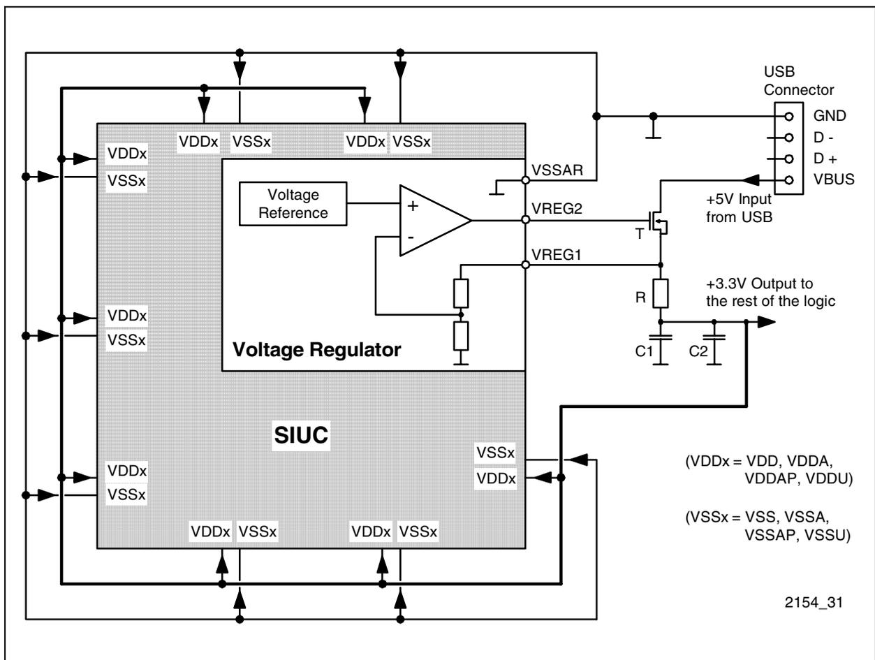
**Figure 135 External Circuitry of the Voltage Regulator**
