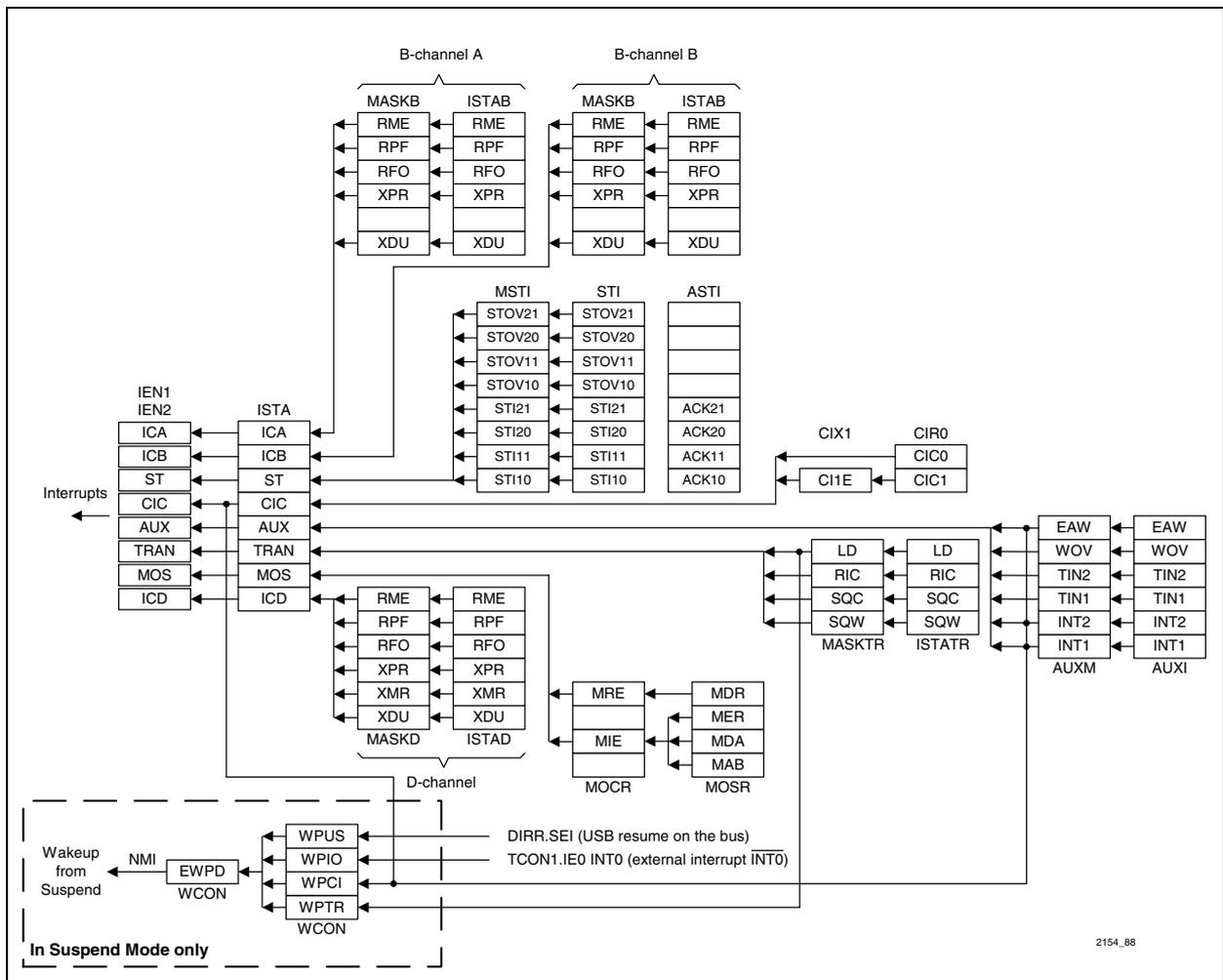
Figure 116 Wakeup Sources in Suspend Mode
