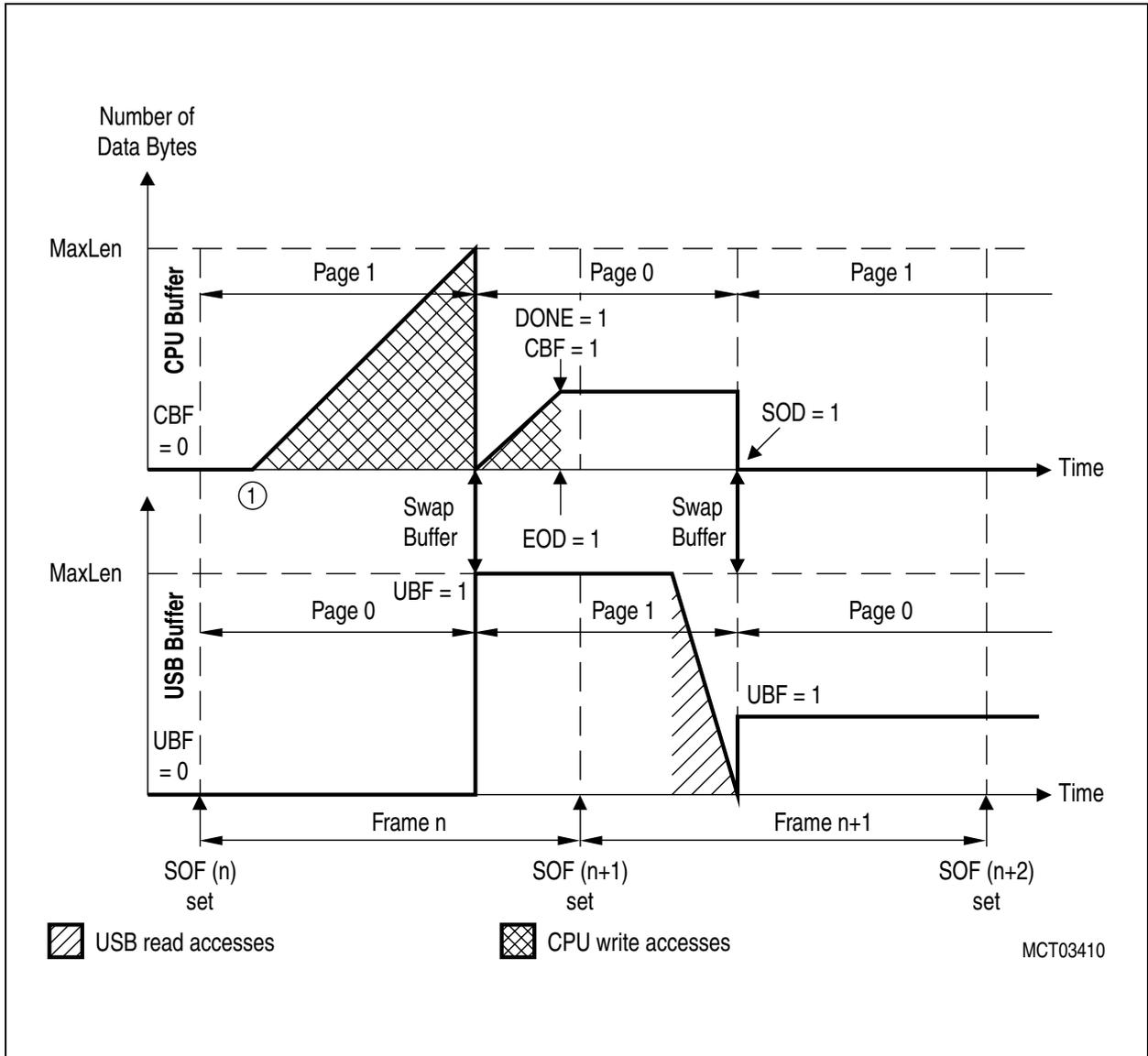
**Figure 36 Double Buffer Mode USB Read Access:
