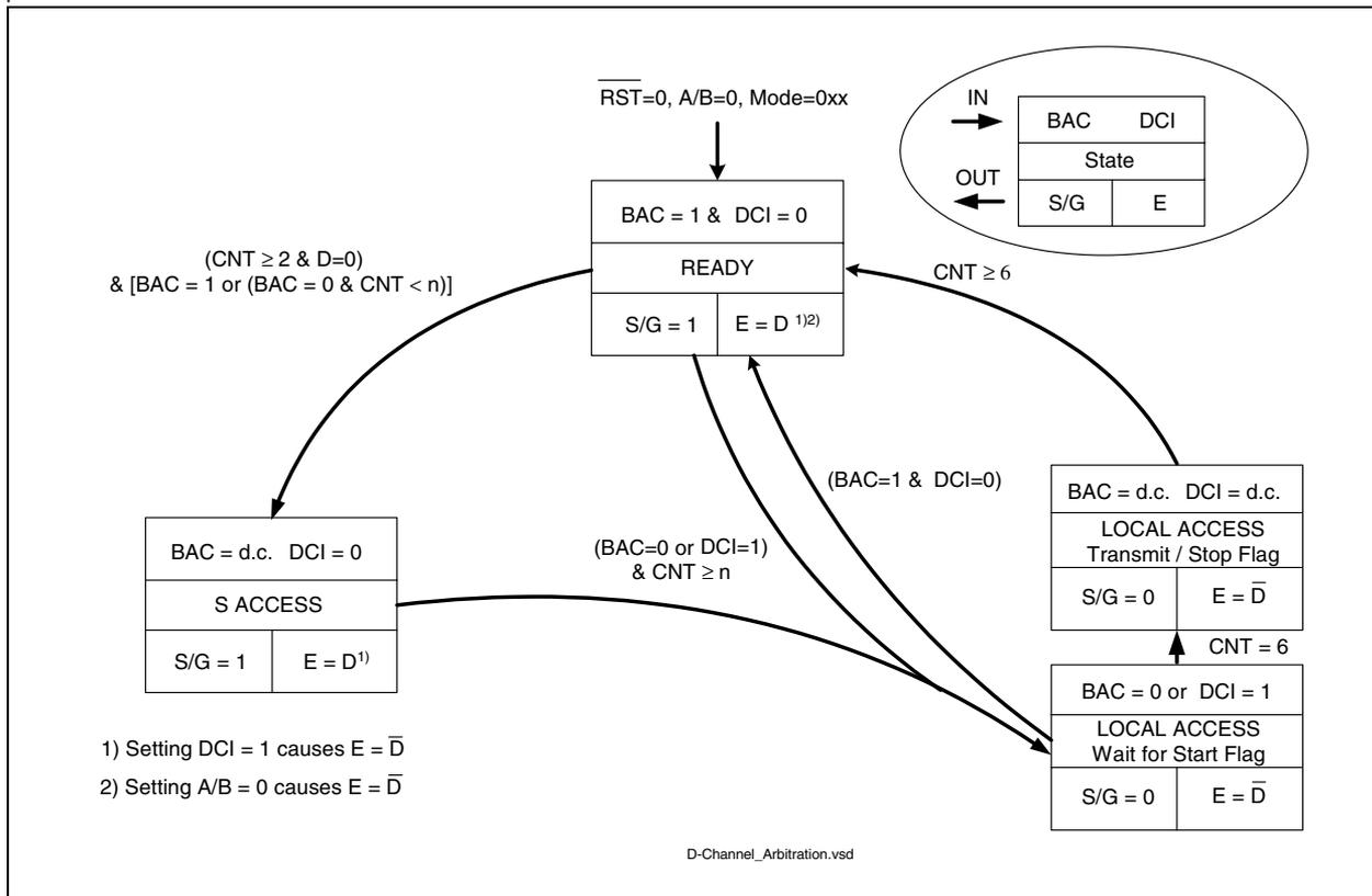
**Figure 98 State Machine of the D-Channel Arbiter (Simplified View)**
