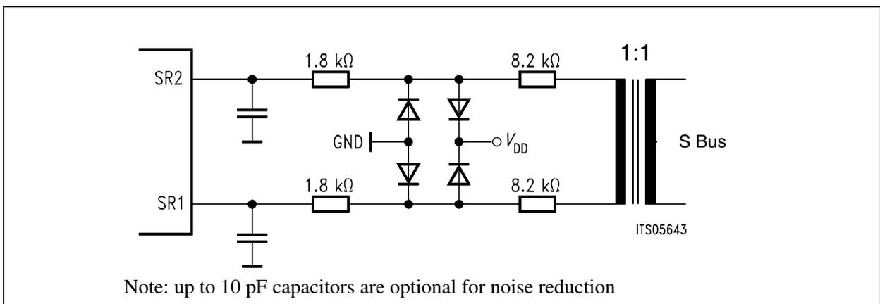
**Figure 62 External Circuitry for Symmetrical Receivers**
