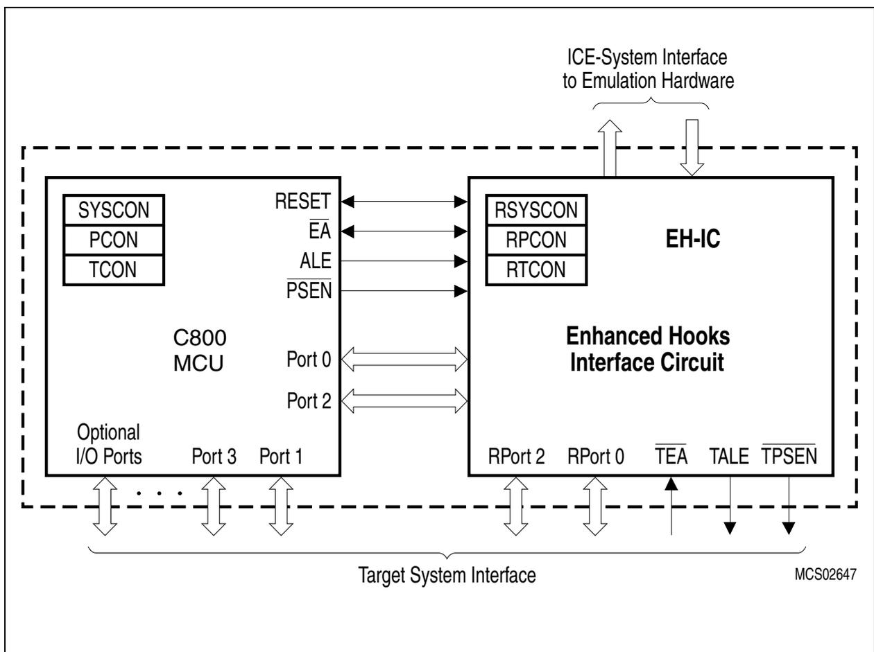
**Figure 18 Basic C800 MCU Enhanced Hooks Concept Configuration**
