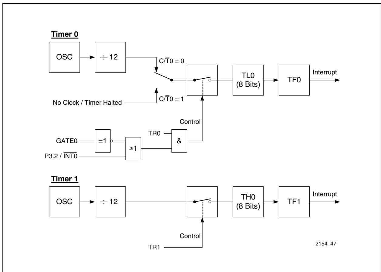
**Figure 22** Timer Mode 3: Two 8-Bit Timers
