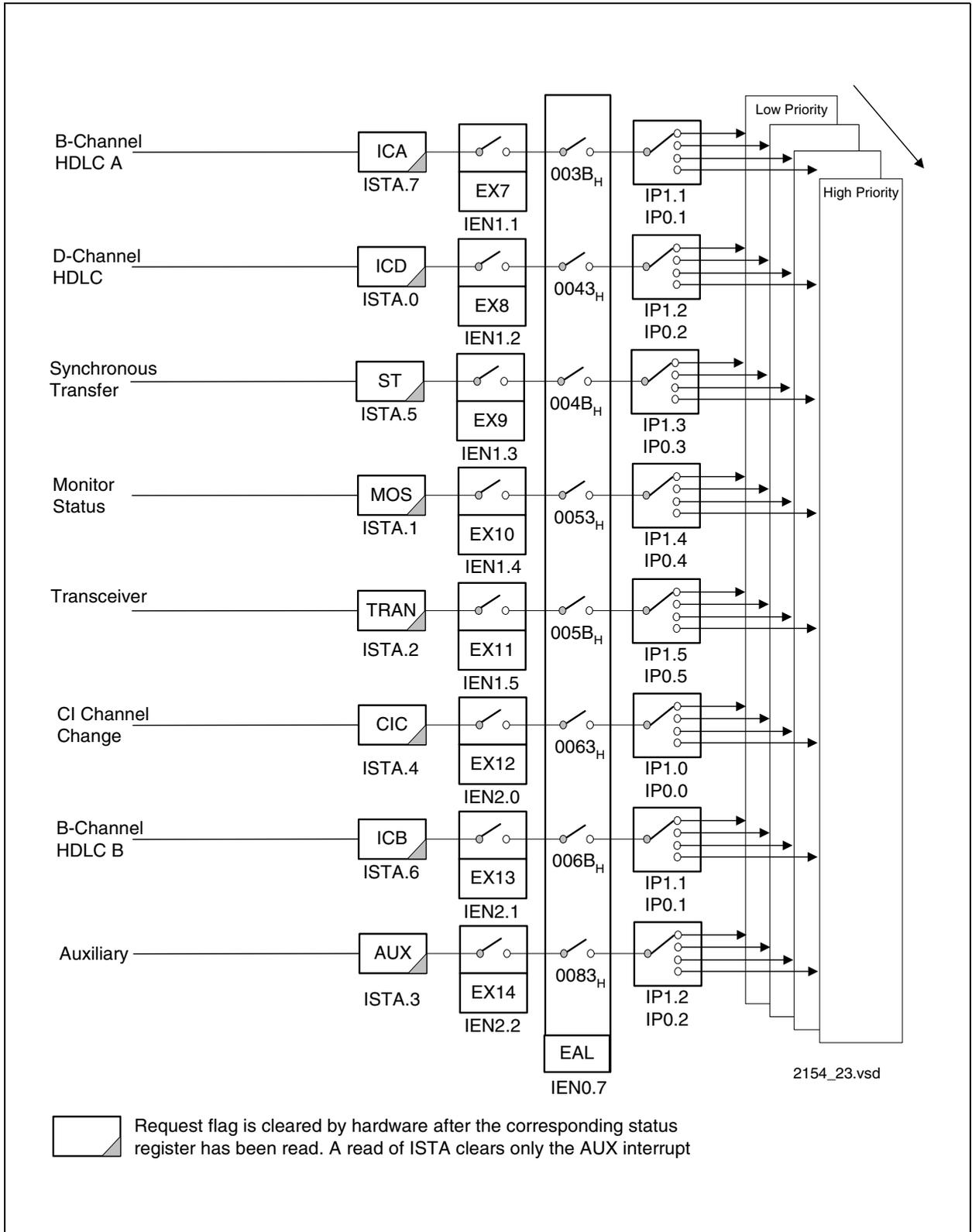
Figure 114 Interrupt Request Sources (Part 4) - ISDN Interrupts
