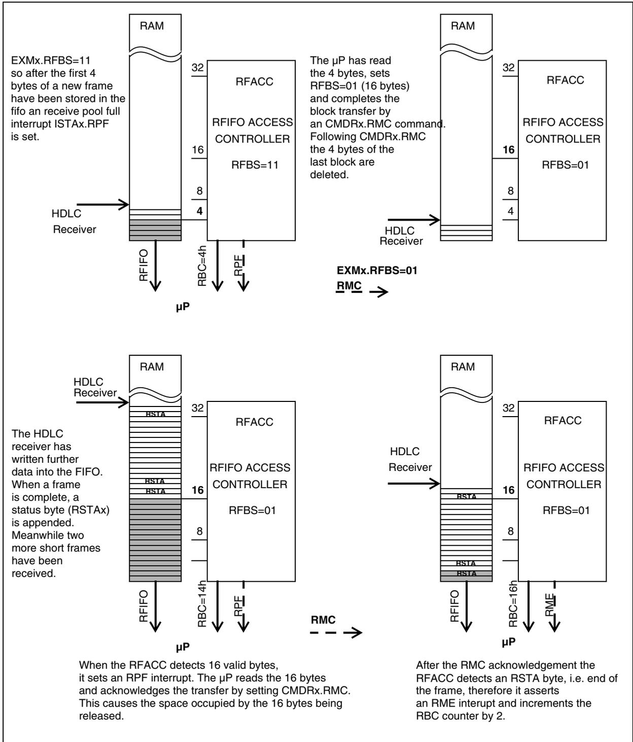
**Figure 101 RFIFO Operation**
