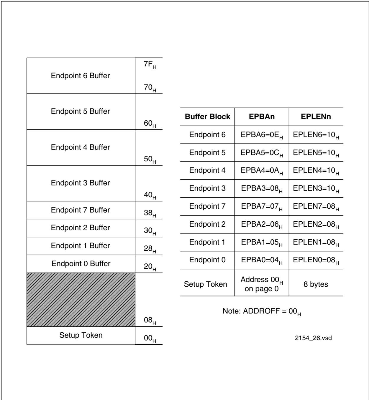
**Figure 37 Endpoint Buffer Allocation (Example: 7+1 Endpoints)**
