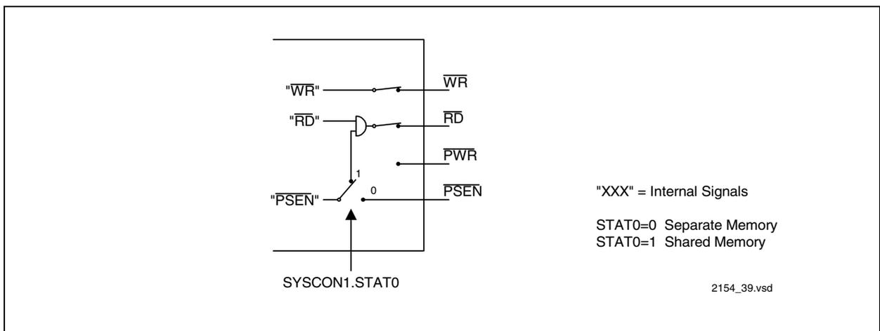
Figure 12 Switching of Read Strobe Signals for Shared Memory
