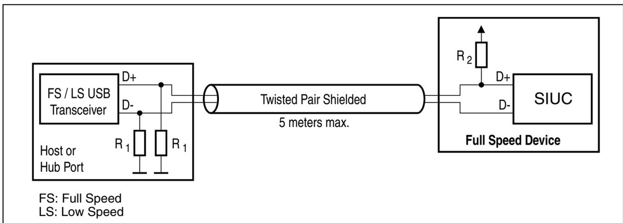
**Figure 41 High Speed Device Cable and Resistor Connection**
