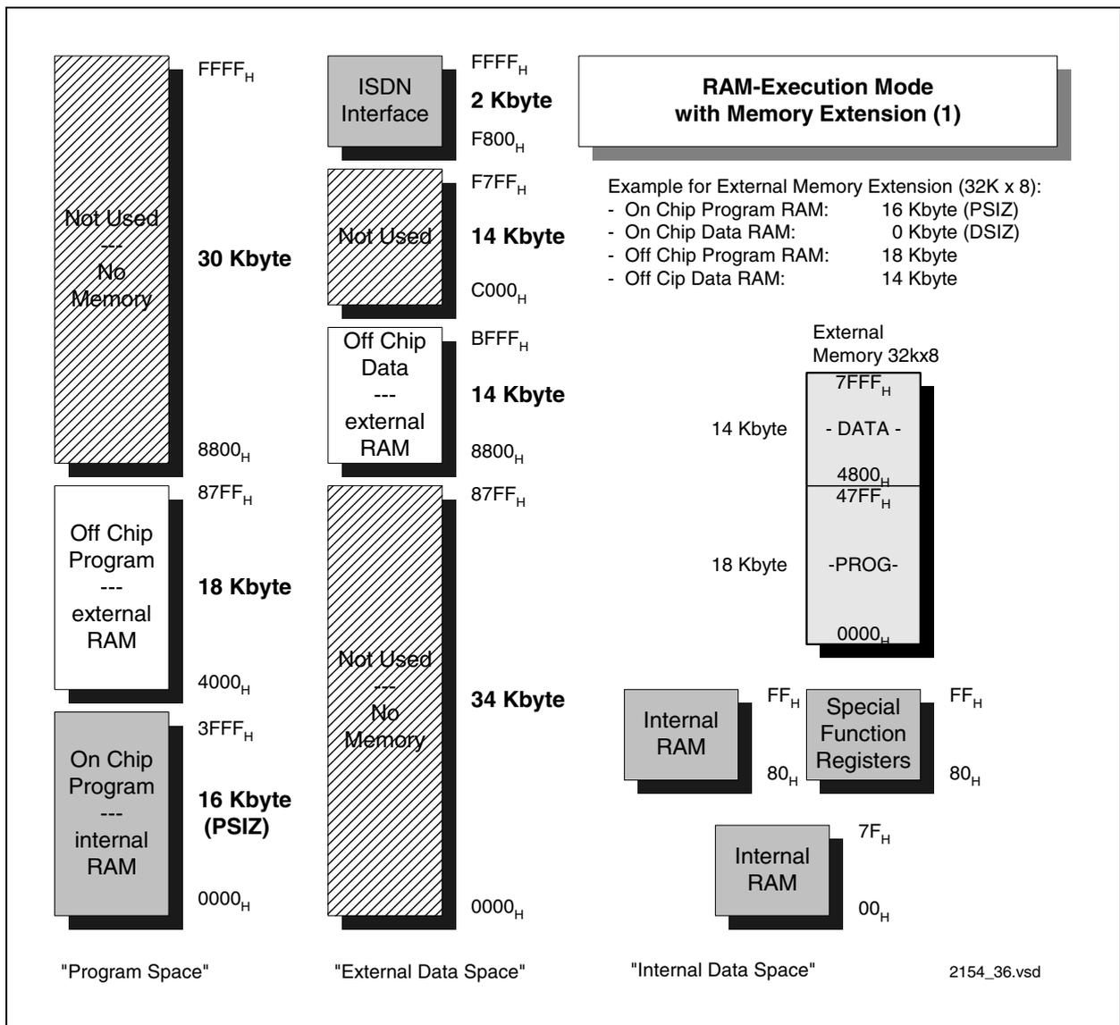
**Figure 122 Firmware Execution in RAM - Example with One 32K Memory**
