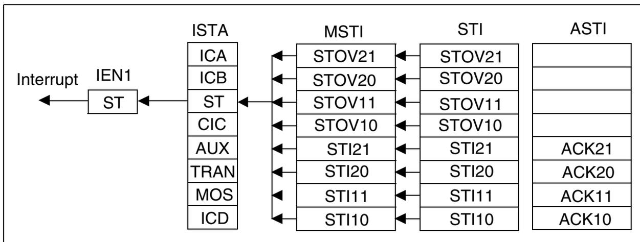
**Figure 79 Interrupt Structure of the Synchronous Data Transfer**
