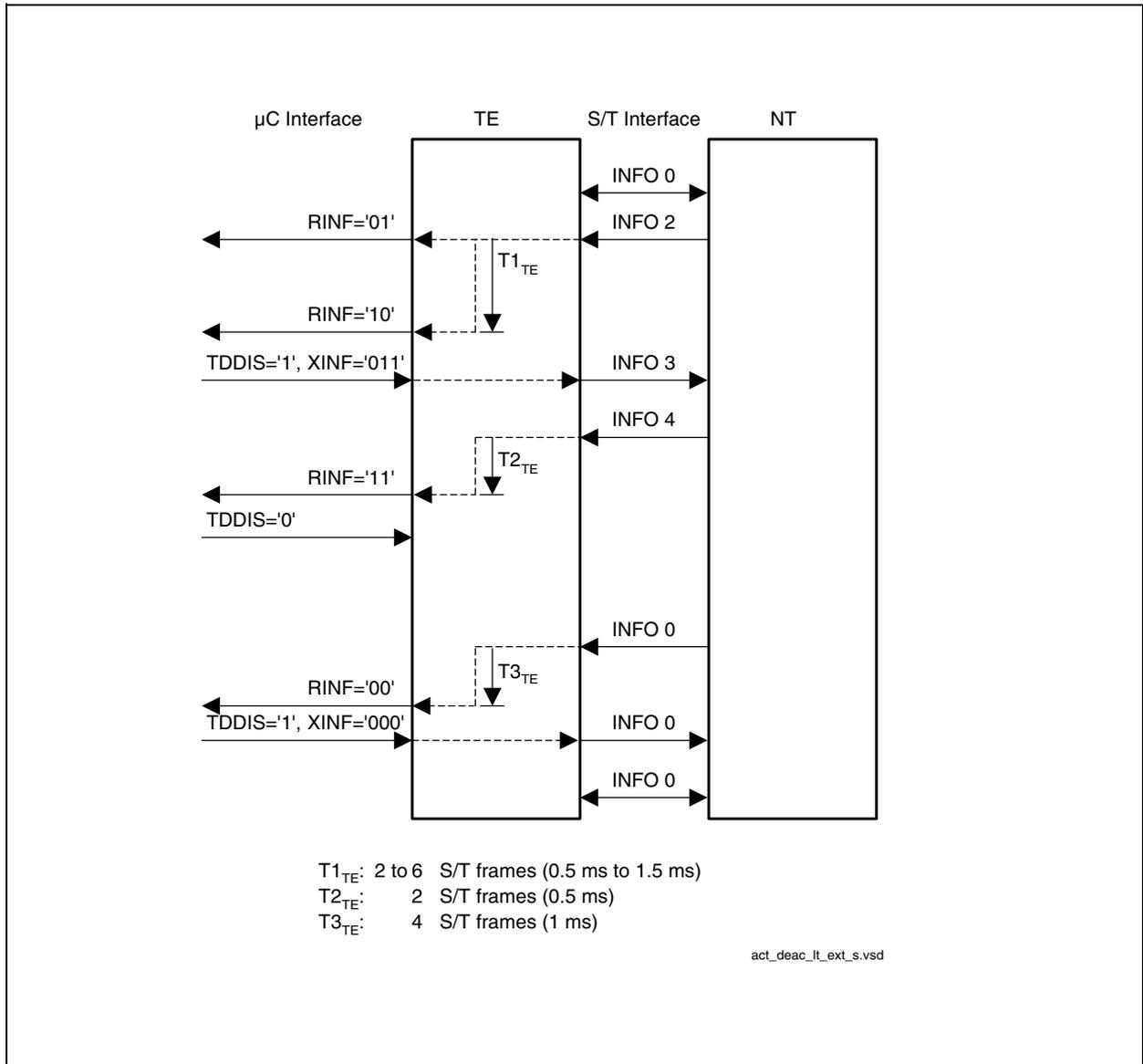
**Figure 71 Example of Activation/Deactivation initiated by the Network Termination (NT).
