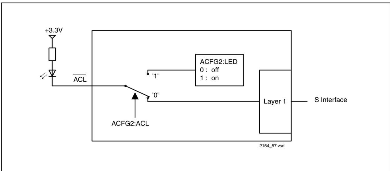
**Figure 50 ACL Configuration**
