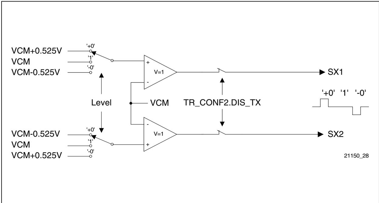
**Figure 58** Equivalent Internal Circuit of the Transmitter Stage
