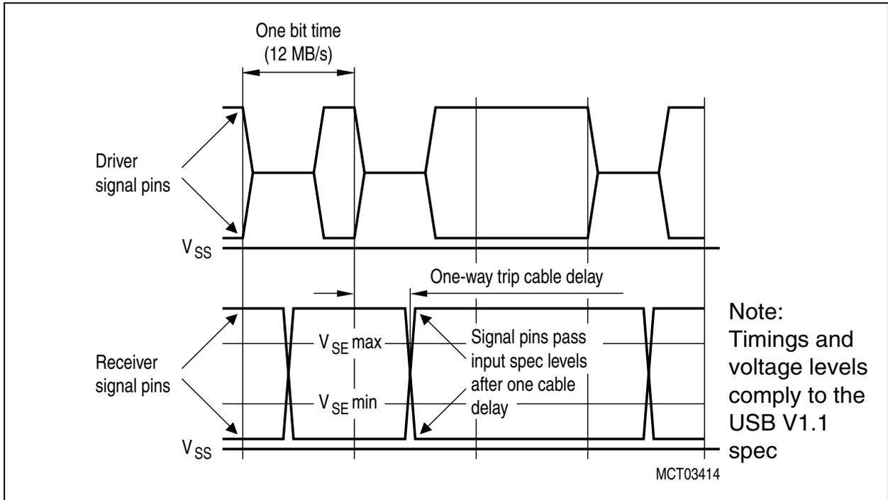
**Figure 40 Full Speed USB Driver Signal Waveforms**
