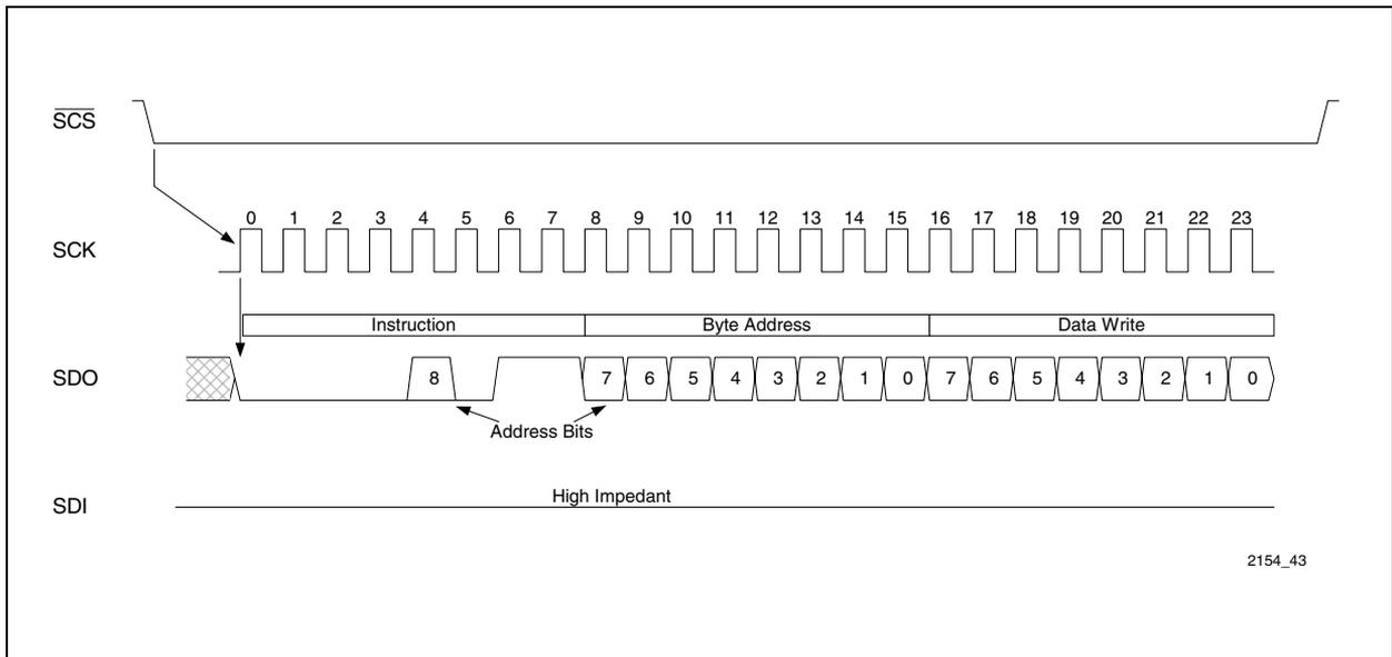
Figure 134 SPI Write Access
