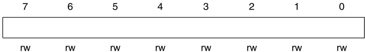
In order to enable ISDN interrupt generation to the microcontroller, the ISTA\_INIT register must be programmed to 00<sub>H</sub> after reset. After that this register should not be changed any more.
