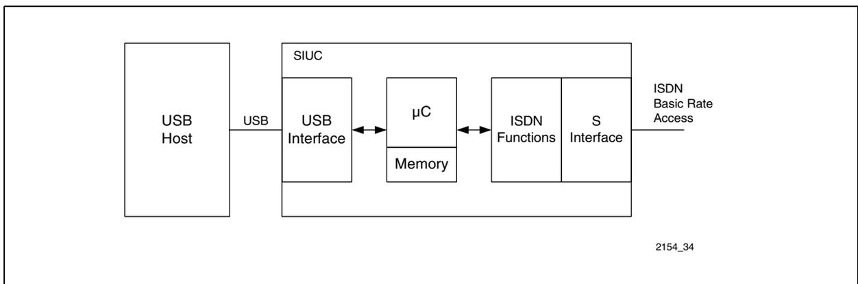
**Figure 128 SIUC-X Firmware Operation**
