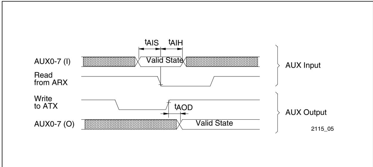
**Figure 148** AUX Interface I/O Timing
