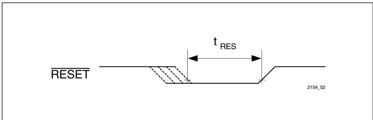
Figure 152 Reset Signal
