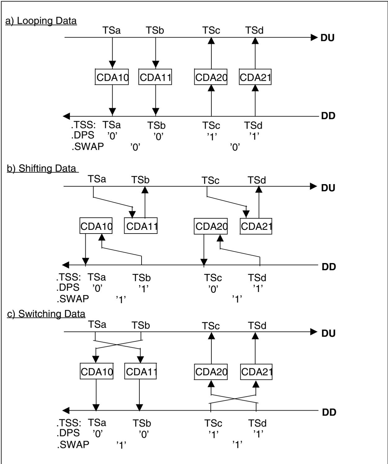
**Figure 75 Examples for Data Access via CDAxy Registers**
