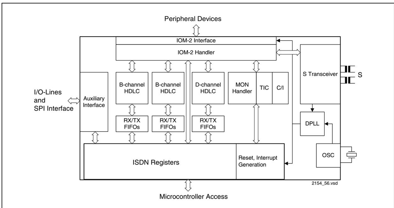
Figure 45 Functional Block Diagram of the SIUC-X
