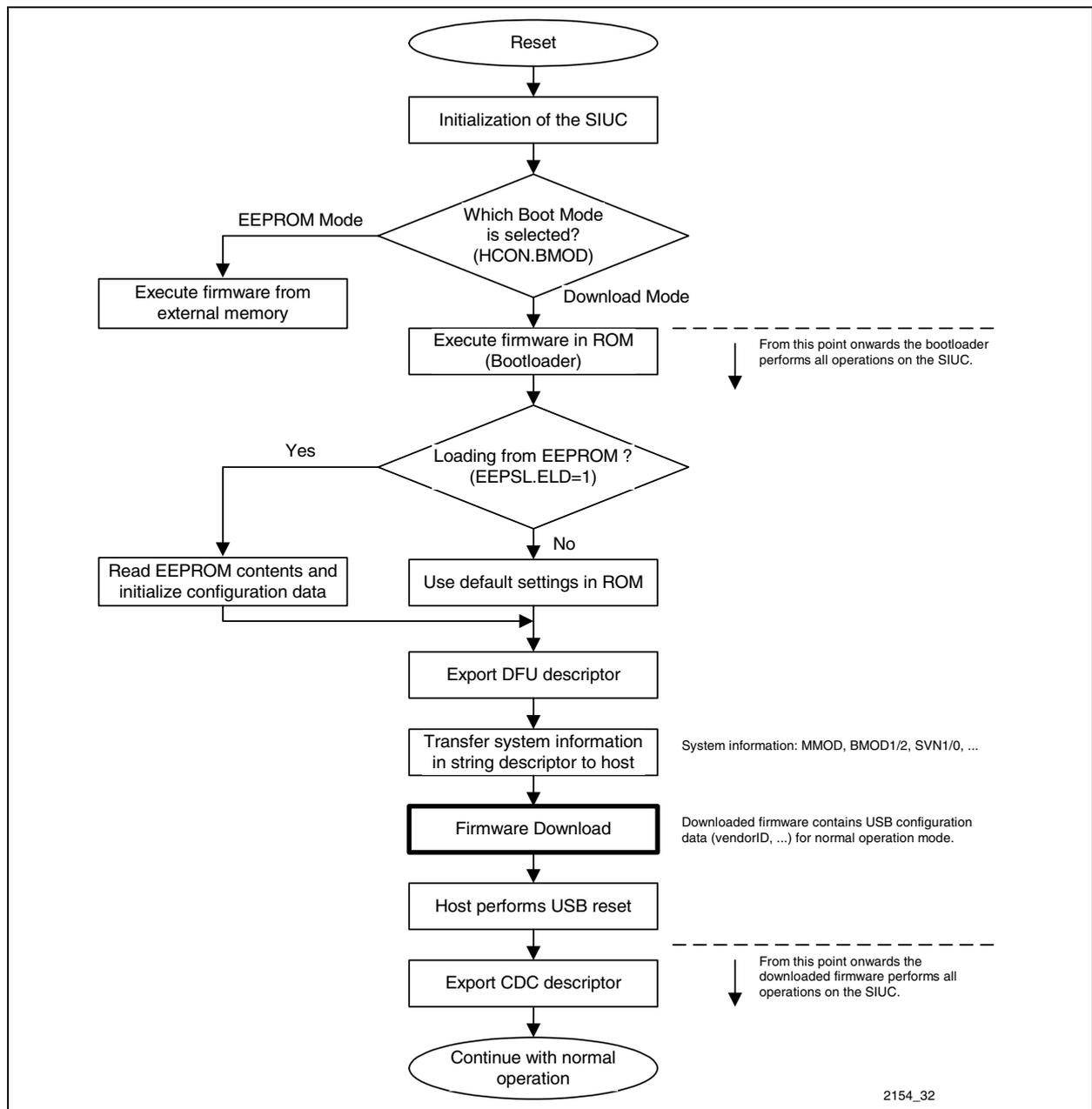
**Figure 117 Bootmode Procedure**
