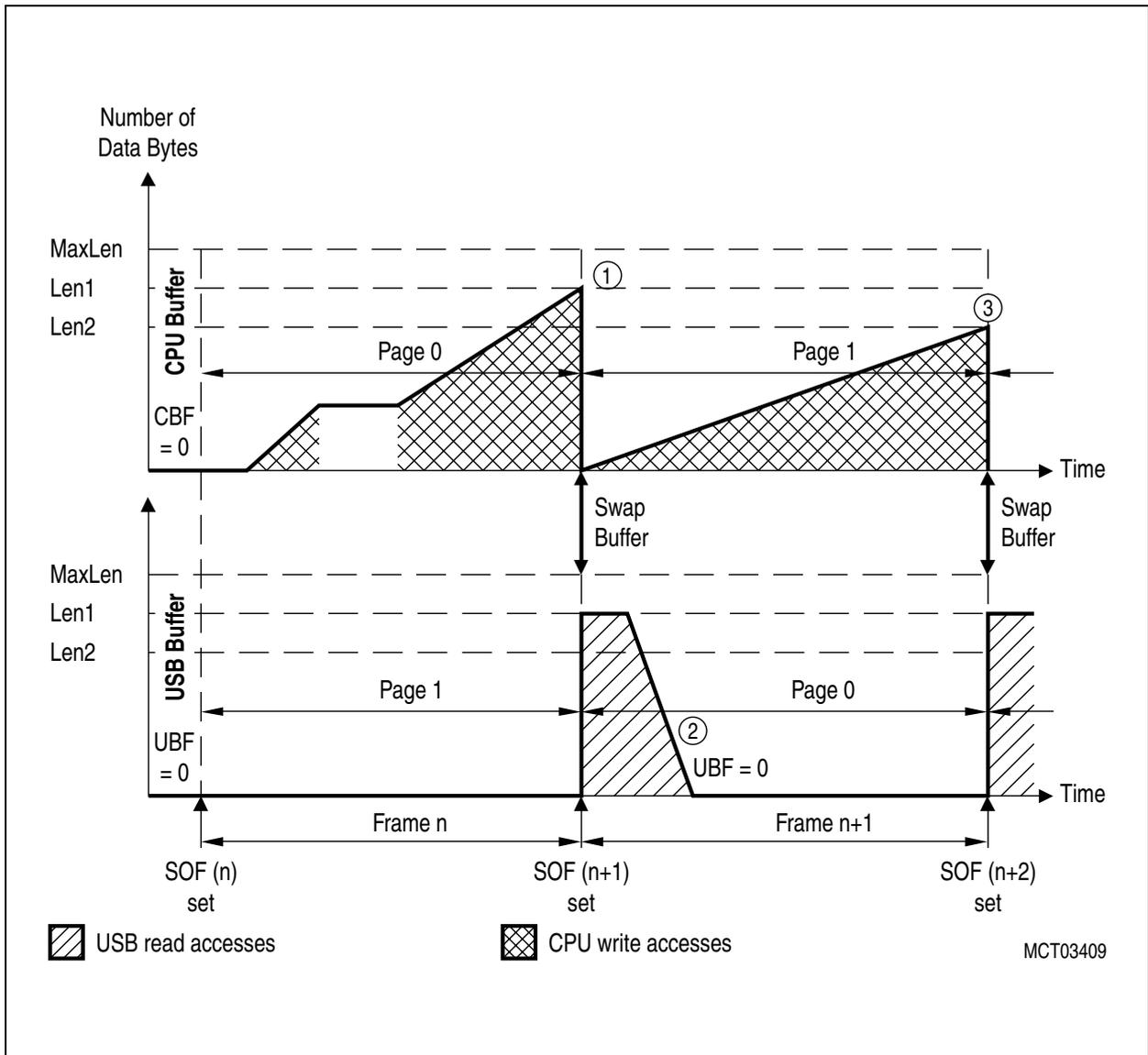
**Figure 35 Dual Buffer Mode USB Read Access: Buffer Switching on SOF with SOFDE=1**
