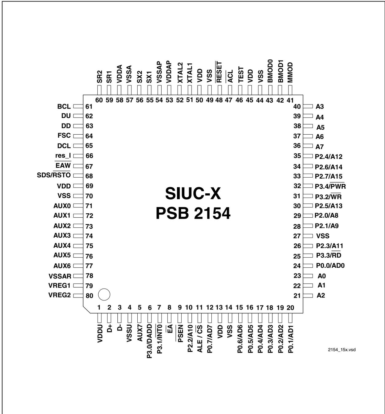
Figure 7 Pin Diagram
