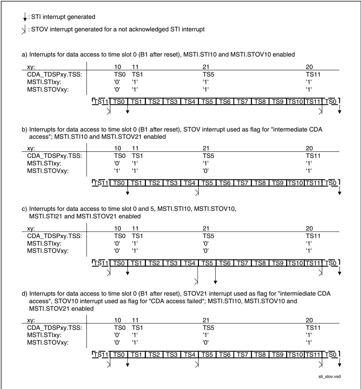
**Figure 80** Examples for the Synchronous Transfer Interrupt Control with one enabled STIxy
