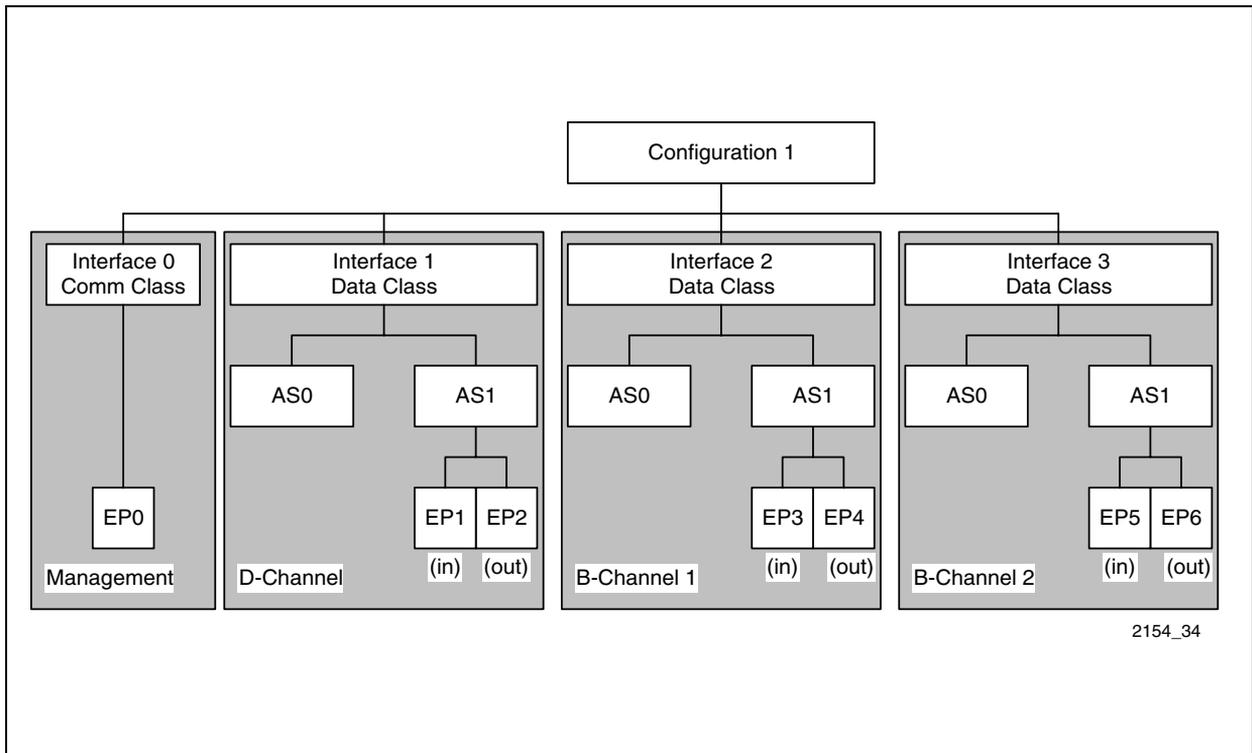
**Figure 129 USB Configuration in CDC Mode**
