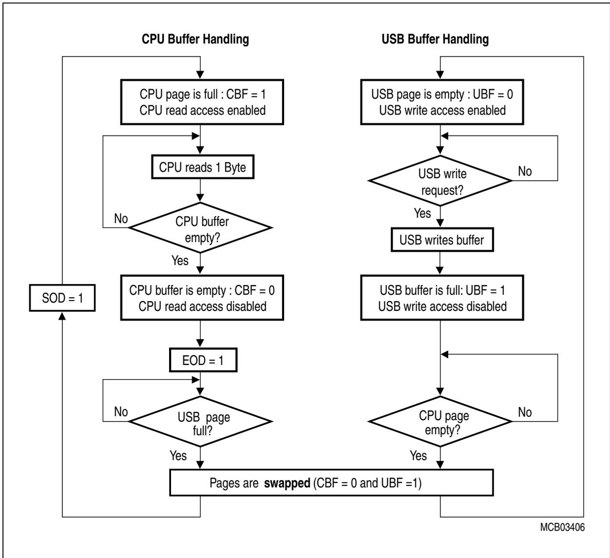
**Figure 32 USB Write Access in Dual Buffer Mode - Buffer Handling**
