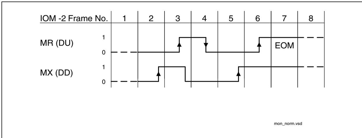
**Figure 91 Monitor Channel, Normal End of Transmission**
