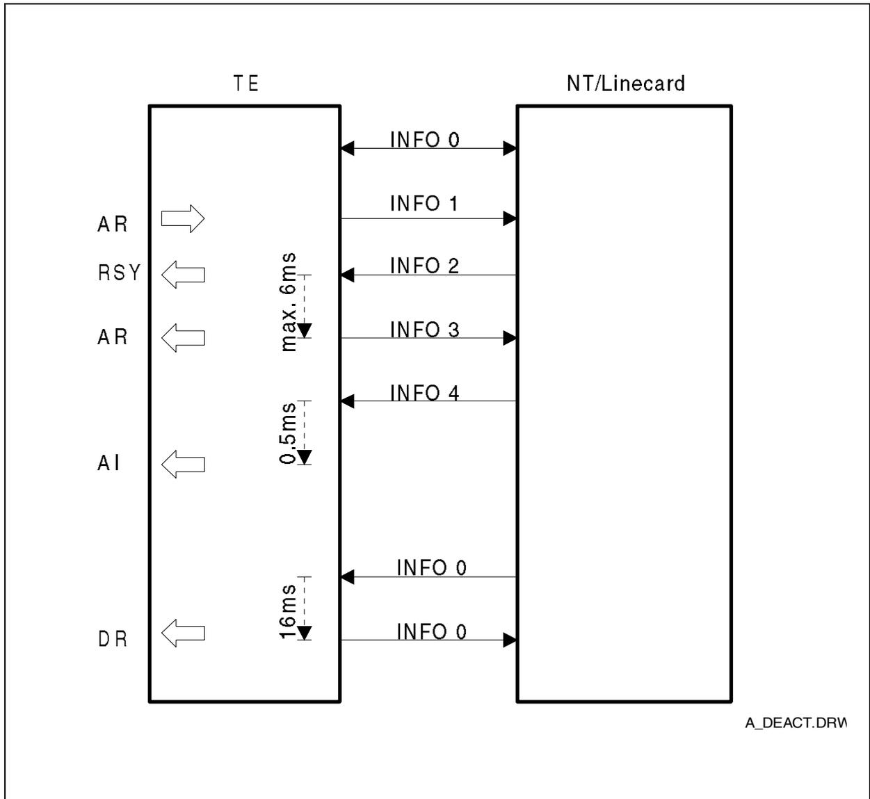
**Figure 69 Example of Activation/Deactivation Initiated by the Terminal**
