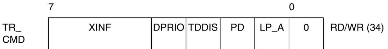
Important: This register is used only if the Layer 1 state machine of the SIUC-X is disabled (TR\_CONFO.L1SW = 1) and implemented in software! With the SIUC-X layer 1 state machine enabled, the signals from this register are automatically generated.
