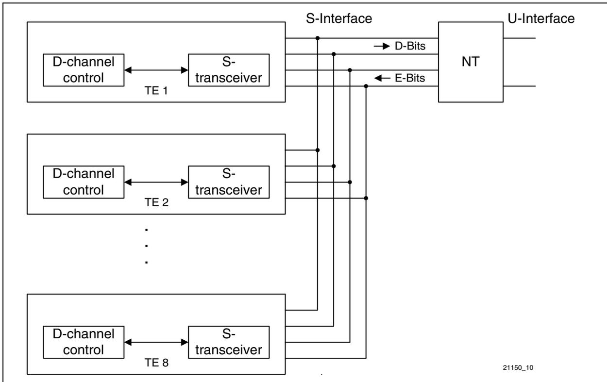
**Figure 97 D-Channel Access Control on the S-Interface**
