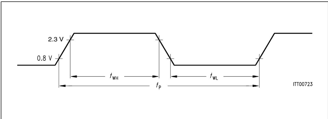
Figure 141 Definition of Clock Period and Width
