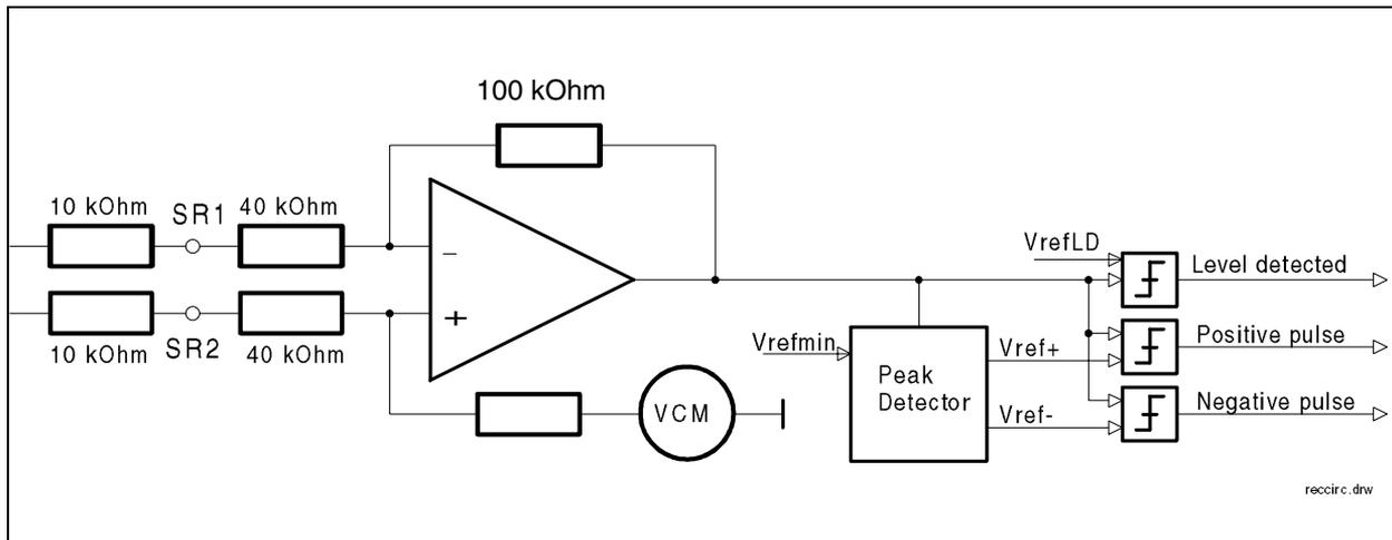
**Figure 59 Equivalent Internal Circuit of the Receiver Stage**
