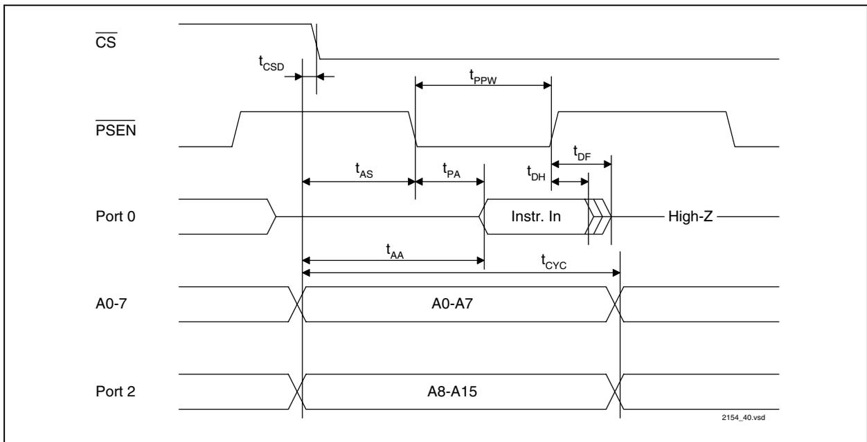
Figure 142 Program Memory Read Cycle - Normal Mode
