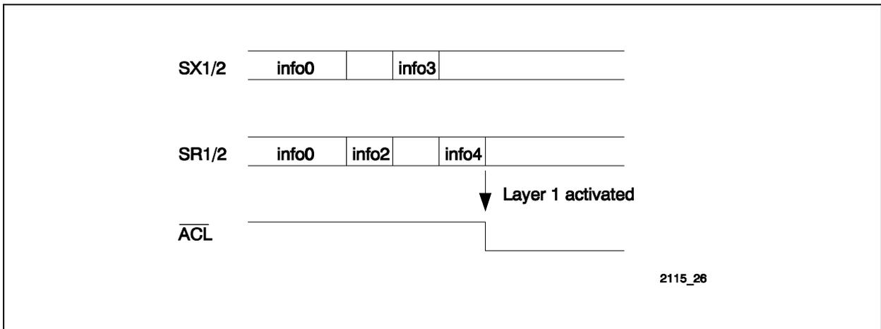
**Figure 49 ACL Indication of Activated Layer 1**
