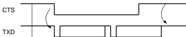
Figure 21-28. Transmitter Behavior when Operating with Hardware Handshaking
