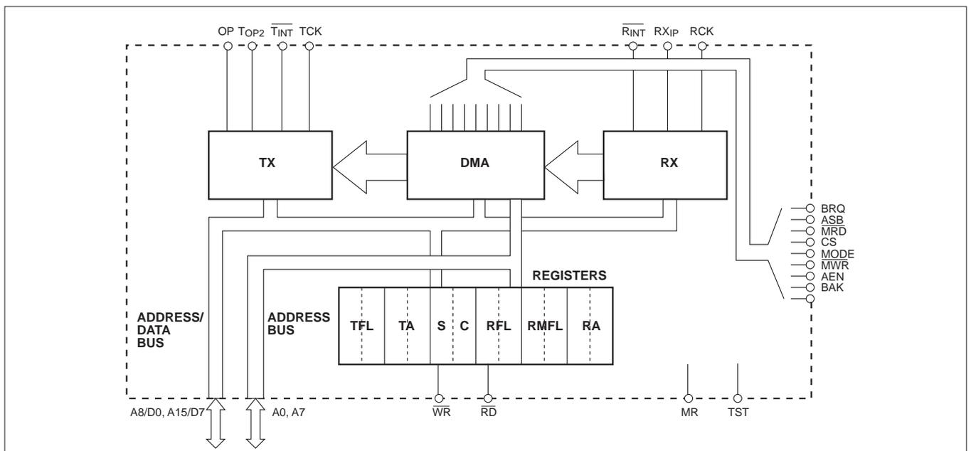
Figure 2: Block diagram
