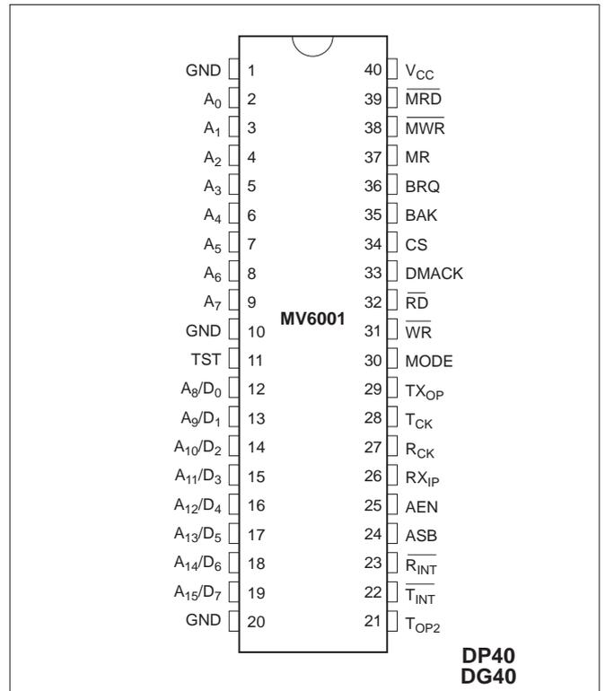
Figure 1: Pin connections - top view
