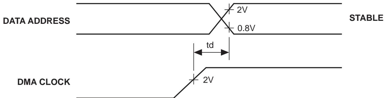
Figure 10: DMA timing
