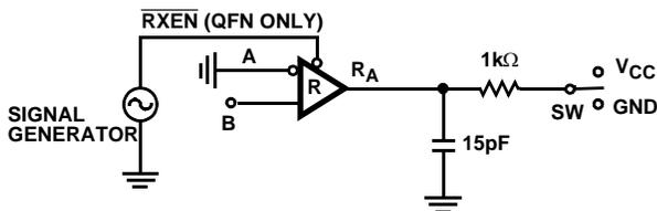
FOR SHDN TESTS, SWITCH ON/OFF RATHER THAN RXEN
