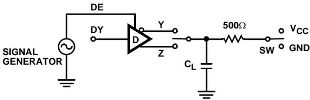
FOR SHDN TESTS, SWITCH ON/OFF RATHER THAN DE
