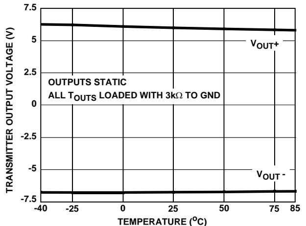
FIGURE 35. RS-232, TRANSMITTER OUTPUT VOLTAGE vs TEMPERATURE
