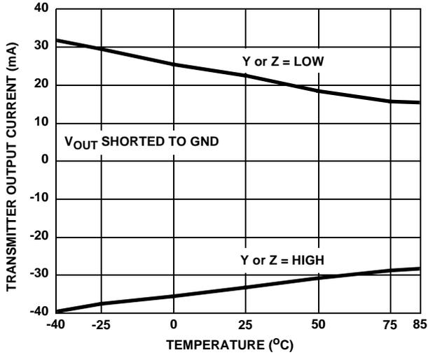
FIGURE 36. RS-232, TRANSMITTER SHORT CIRCUIT CURRENT vs TEMPERATURE
