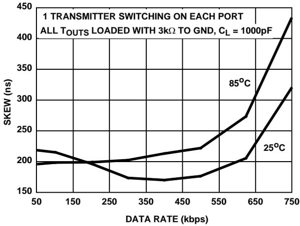
FIGURE 42. RS-232, TRANSMITTER SKEW vs DATA RATE
