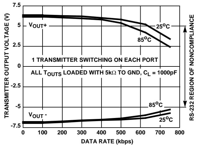
FIGURE 41. RS-232, TRANSMITTER OUTPUT VOLTAGE vs DATA RATE
