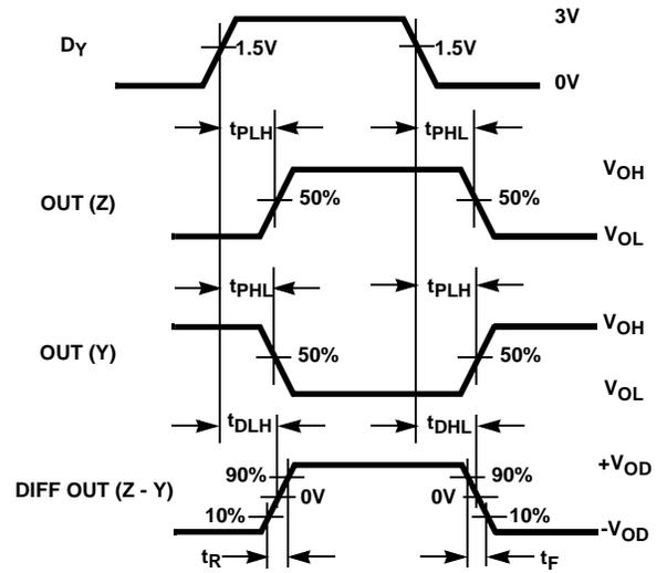
$$\text{SKEW} = |t_{PLH}(Y \text{ or } Z) - t_{PHL}(Z \text{ or } Y)|$$
