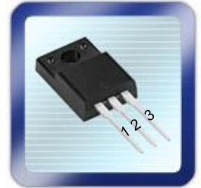
T0220 Full-PAK Isolated (T0-220) 1=Gate, 2=Drain, 3=Source
