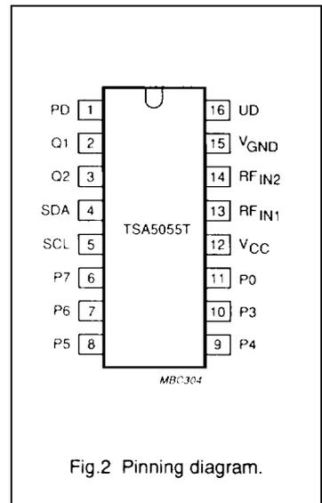
Fig.2 Pinning diagram.
