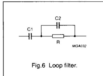
Fig.6 Loop filter.
