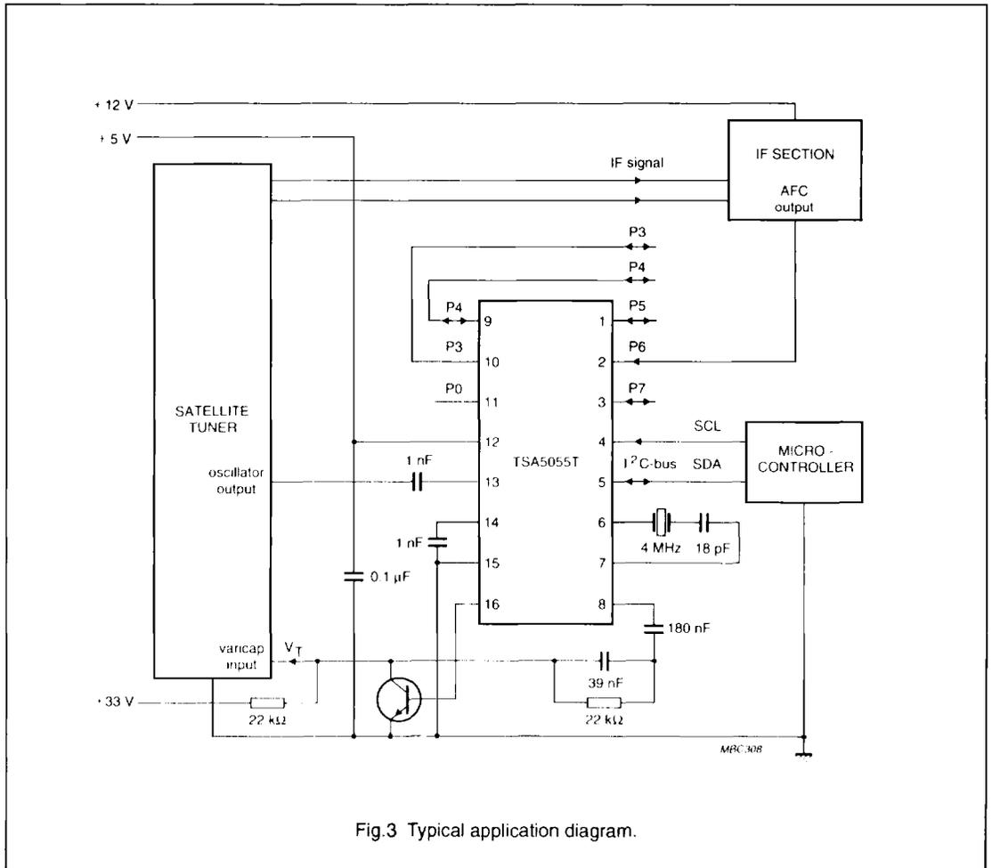
Fig.3 Typical application diagram.
