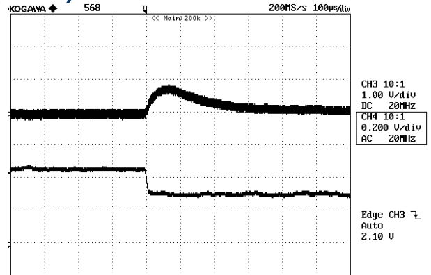
Figure 8: Output voltage response to step-change in load current (75%-50% of I_o , max; di/dt = 0.1A/\mu s ). Load cap: 10µF tantalum capacitor and 1µF ceramic capacitor. Top Trace: V_{out} (200mV/div, 100µs/div), Bottom Trace: I_{out} (1A/div). Scope measurement should be made using a BNC cable (length shorter than 20 inches). Position the load between 51 mm to 76 mm (2 inches to 3 inches) from the module.
