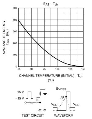
$$\begin{aligned} R_G &= 25~\Omega \\ V_{DD} &= 90~V,~L = 5.73~mH \end{aligned} \qquad E_{AS} &= \frac{1}{2} \cdot L \cdot I^2 \cdot \left( \frac{BVDSS}{BVDSS - VDD} \right) \end{aligned}$$
