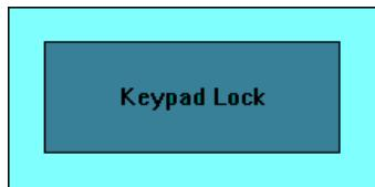
To release the OSD lock, press “Menu” and “Right >”. The below icon will appear on the center of the screen for 3 seconds. Now all OSD keys are active again.
