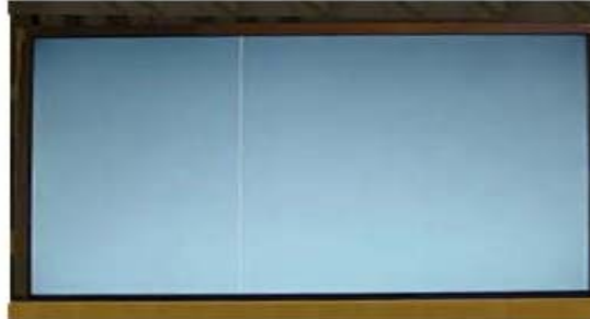
Vertical Line Source TAB IC Defect
