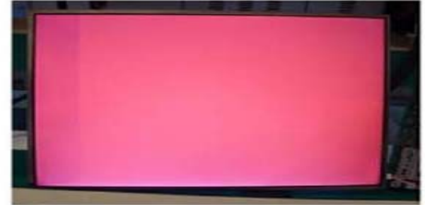
Vertical Block Source TAB IC Defect
