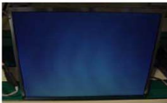
Panel Mura, Light leakage
