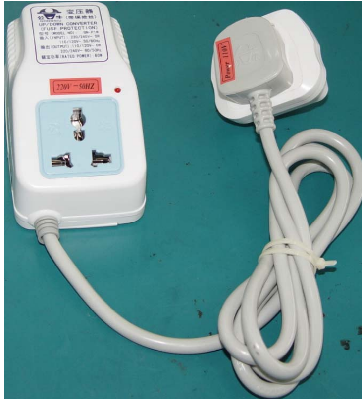
Fig 8 Power switcher from 110V to 220V for visual camera power
