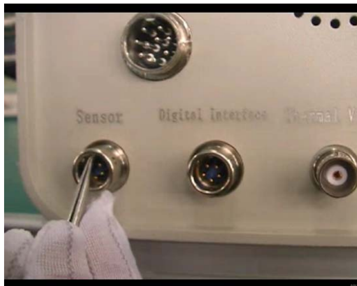
Fig 3. The small gap on the “Sensor” interface
