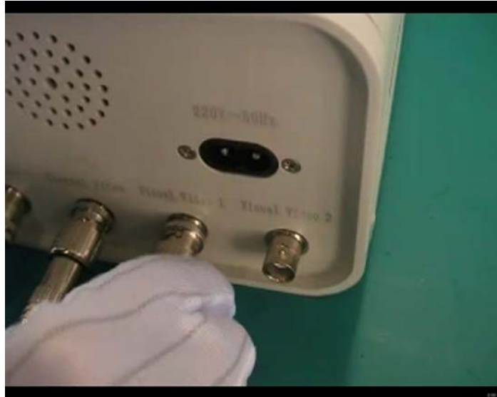
Fig 2. Aim the connector at the interface, press and rotate the connector until it reaches the correct position.
