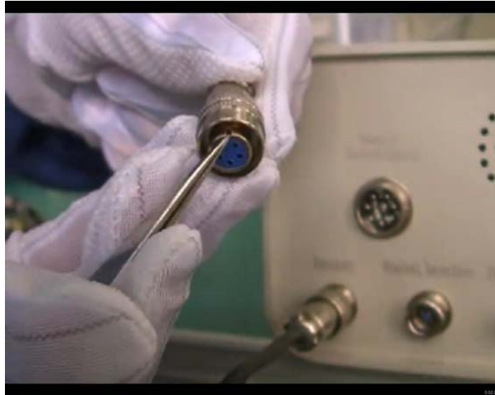
Fig 2. Please notice there is a small gap on the “Digital Interface” connector, which needs to be aimed at the gap in “Digital Interface” on the camera body.
