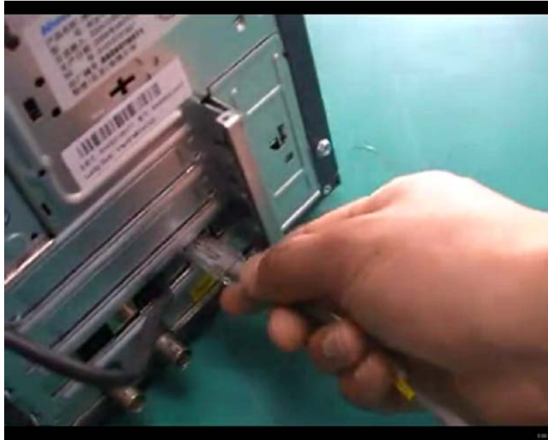
Fig 3 Connect RJ45 connector to the network interface on 1801A card
