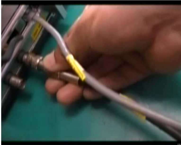
Fig 5 Connect the head of Thermal Video cable onto the “Thermal Video” interface of VT120 card
