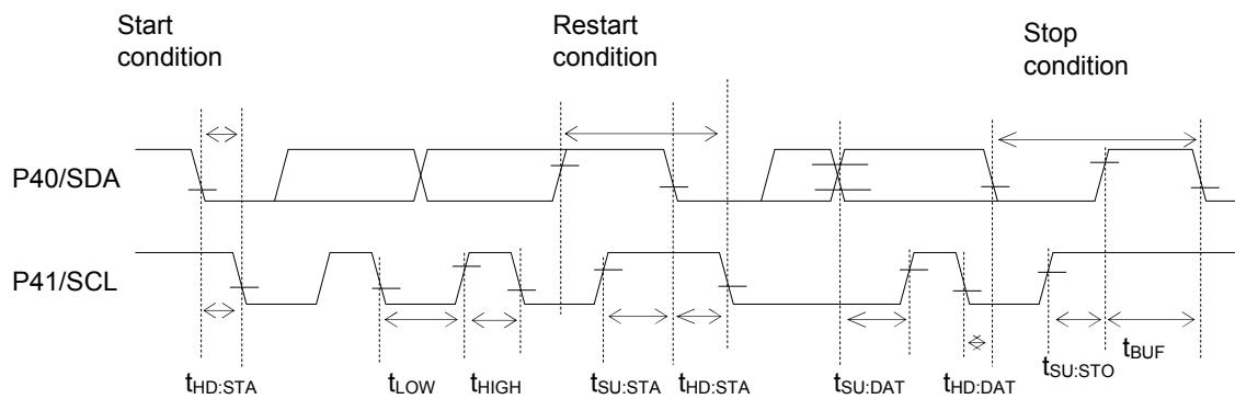
**AC CHARACTERISTICS (RC Oscillation A/D Converter)**
