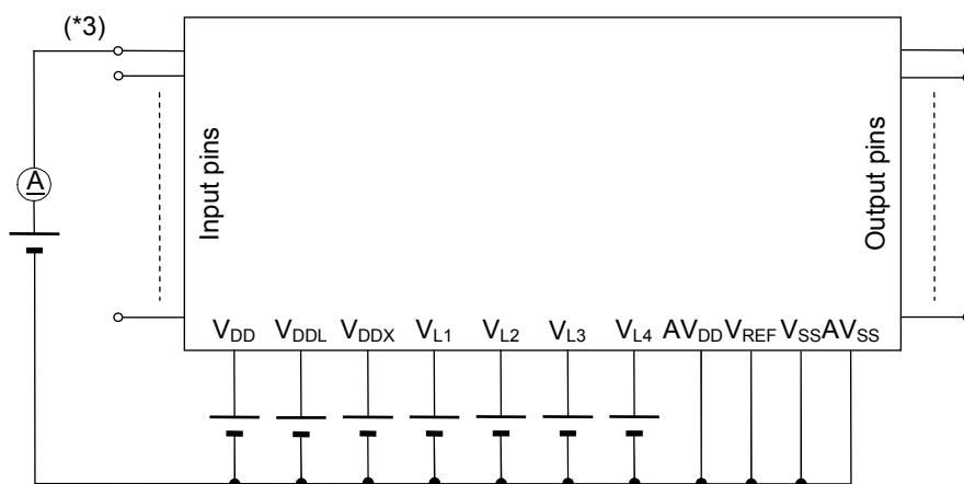
\*3: Measured at the specified output pins.
