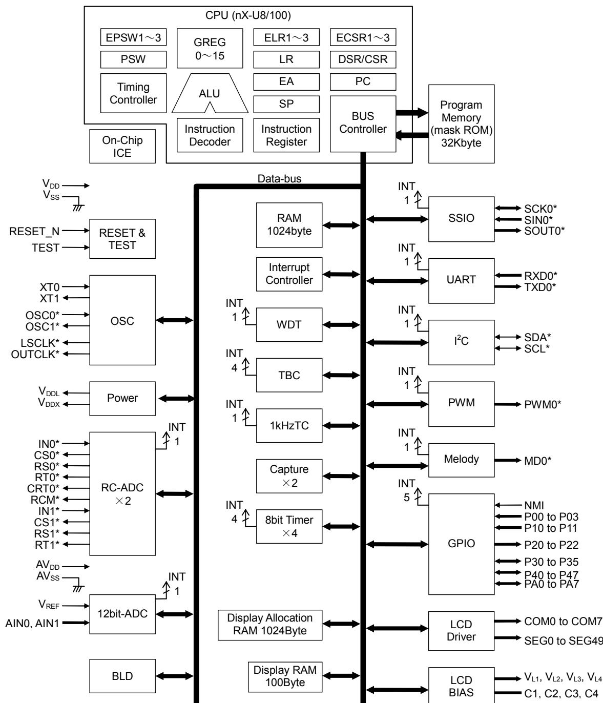
Figure 1 ML610421 Block Diagram
