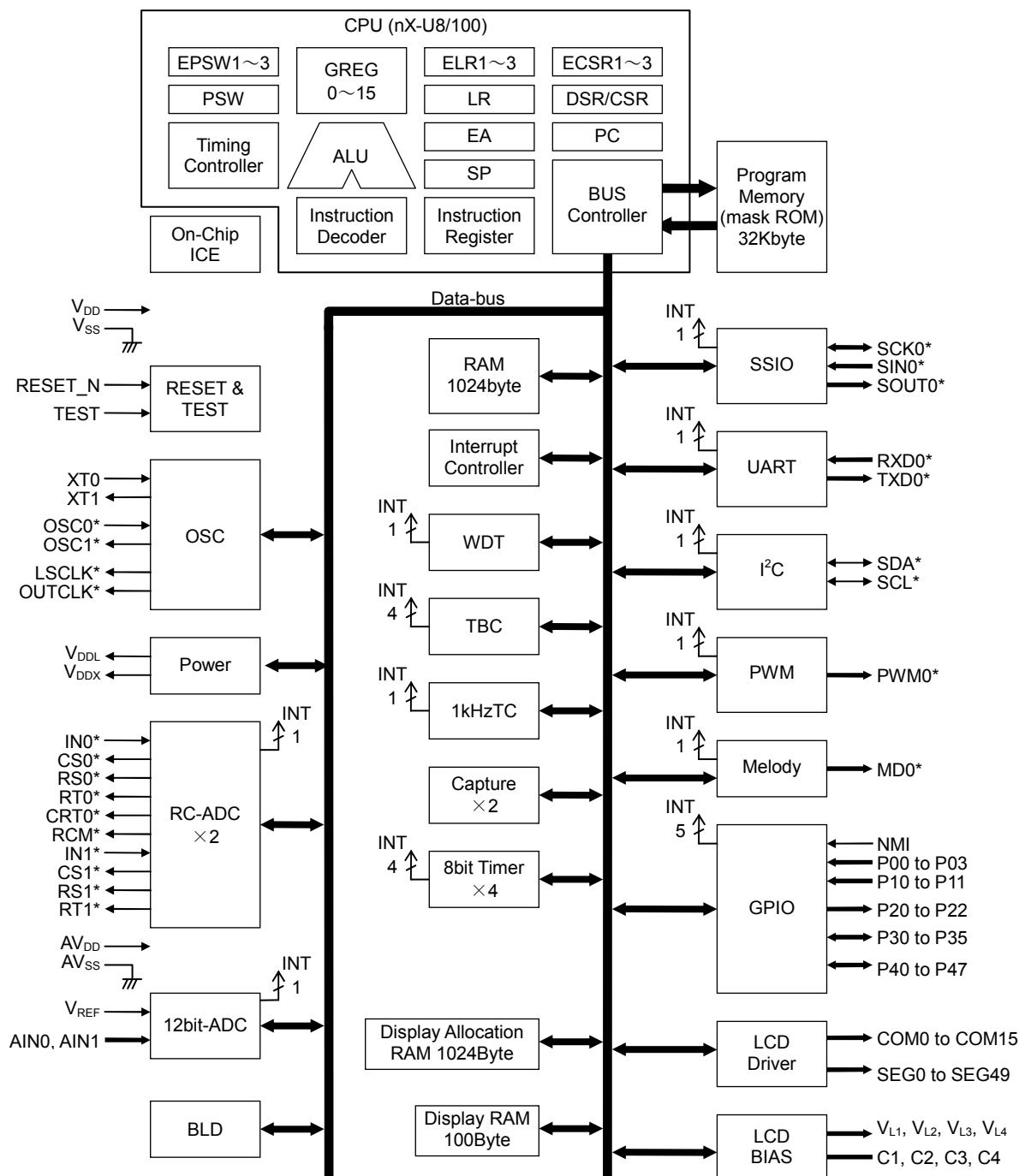
Figure 2 ML610422 Block Diagram
