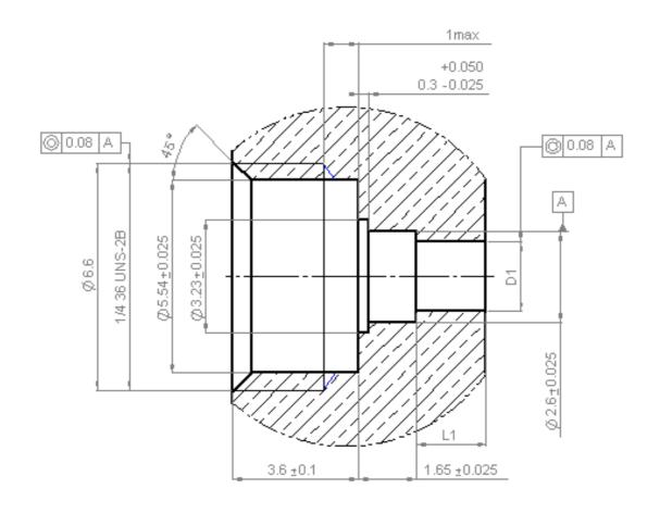
THE D1 AND L1 DIMENSIONS HAVE TO BE DETERMINED ACCORDING TO EACH USING SITUATION WE ADVISE IN THE TWO FOLLOWING SITUATIONS : (SEE PAGE 4/4)
