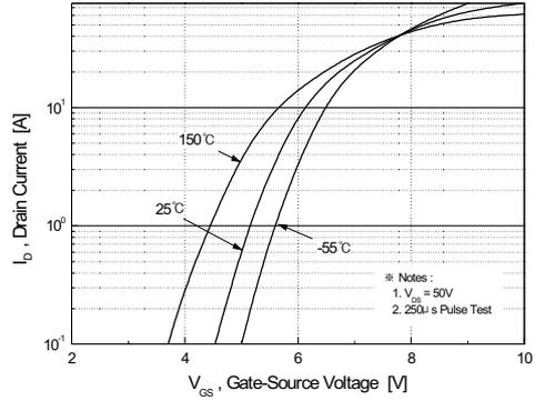
Figure 2. Transfer Characteristics
