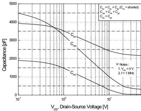
Figure 5. Capacitance Characteristics
