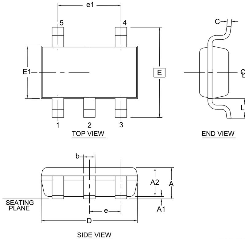
1. Dimension D does not include mold flash, protrusions or gate burrs. Mold flash, protrusions or gate burrs shall not exceed 0.15 mm per end. Dimension E1 does not include interlead flash or protrusion. Interlead flash or protrusion shall not exceed 0.15 mm per side.
