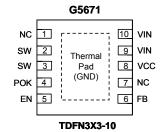
Note: Recommend connecting the Thermal Pad to the Ground for excellent power dissipation.
