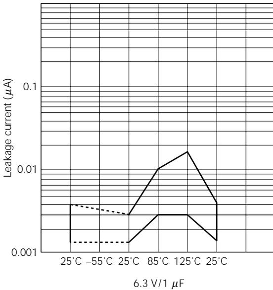
Resistance to soldering (immersing for 10 sec. at 260°C)
