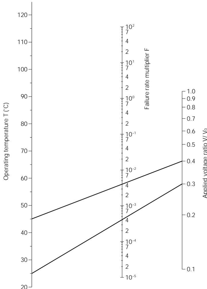
The nomograph is provided for quick estimation of maximum field failure rates.
