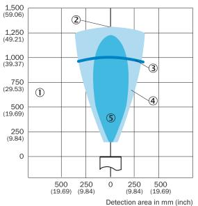
① Sensing range dependent on reflection properties, size and orientation of the object
