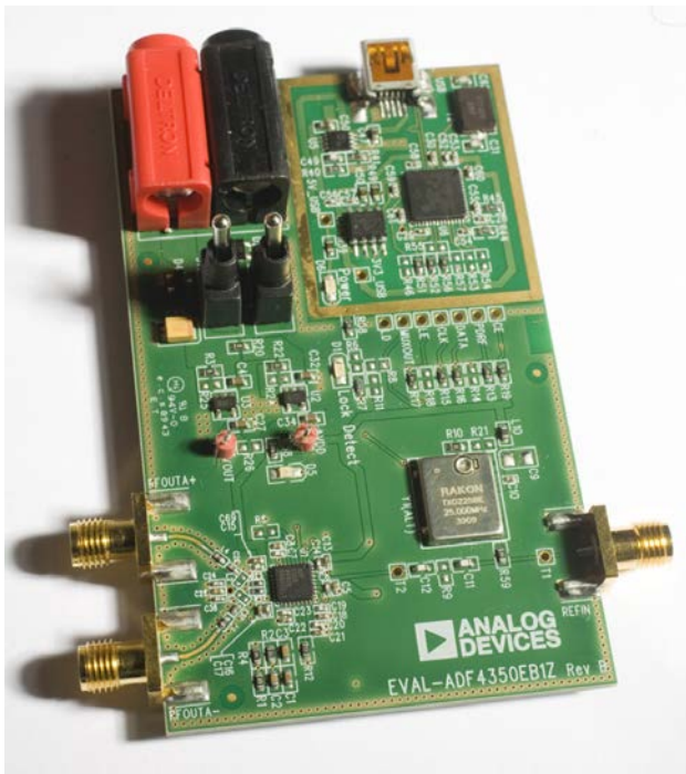
Figure 2. EVAL-ADF4350EB1Z Rev. B Evaluation Board Featuring ADP150 Low Noise Regulators
