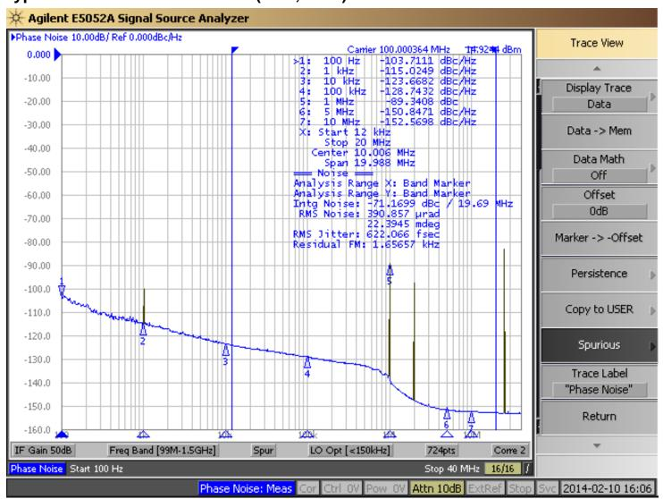
NOTE: All outputs operational at 100MHz, Phase Noise Plot with Spurs On.
