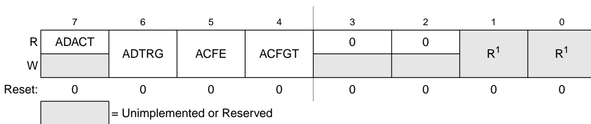
Figure 9-5. Status and Control Register 2 (ADCSC2)
