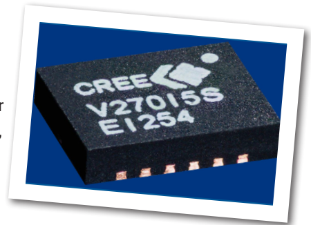
Package Type: 3x4 DFN PN: CGHV27015S
