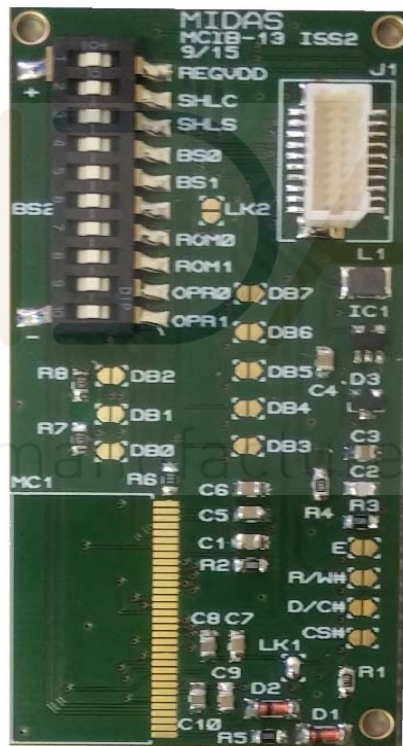
Figure 1. MCIB-13 Interface Board
