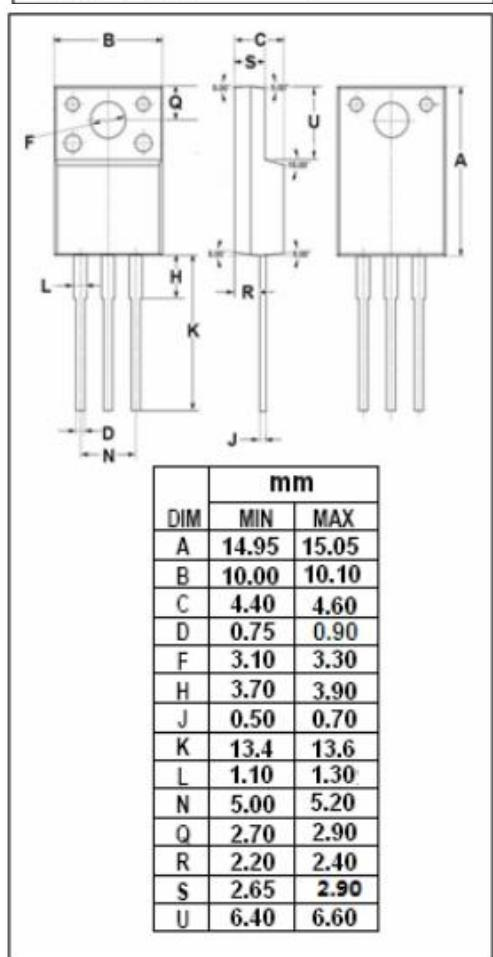
**iscN-Channel MOSFET Transistor      TK14A65W5, ITK14A65W5****ELECTRICAL CHARACTERISTICS** $T_c=25^\circ\text{C}$  unless otherwise specified
