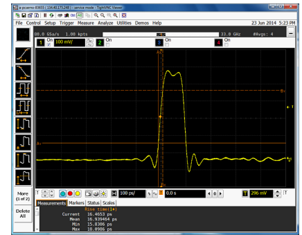
Figure 5. 100 ps pulse with 17 ps risetime.
