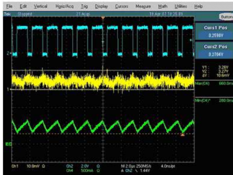
Figure 9. Ceramic 22 \mu F 1210 (X5R) (Good)
