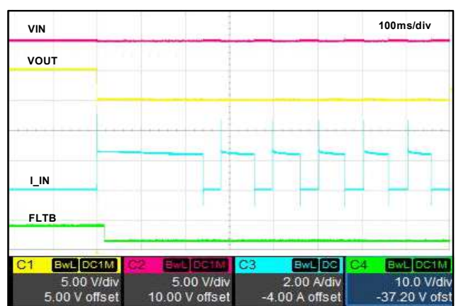
Figure 9. Short Circuit Protection, Thermal Shutdown (Auto Restart)
